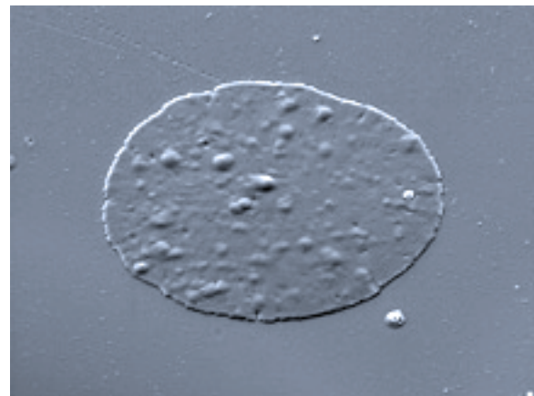
Figure 5. Scanning Electron Microscope: Image of ink dot on overhead transparency (1000 ×)
