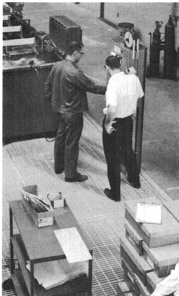
PANELS ARE SPOTTED to cover defects in the photo resist coating; from here they go to detail etching area (left). Control panel for automatic anodizing machine gets final check before production starts (right).
