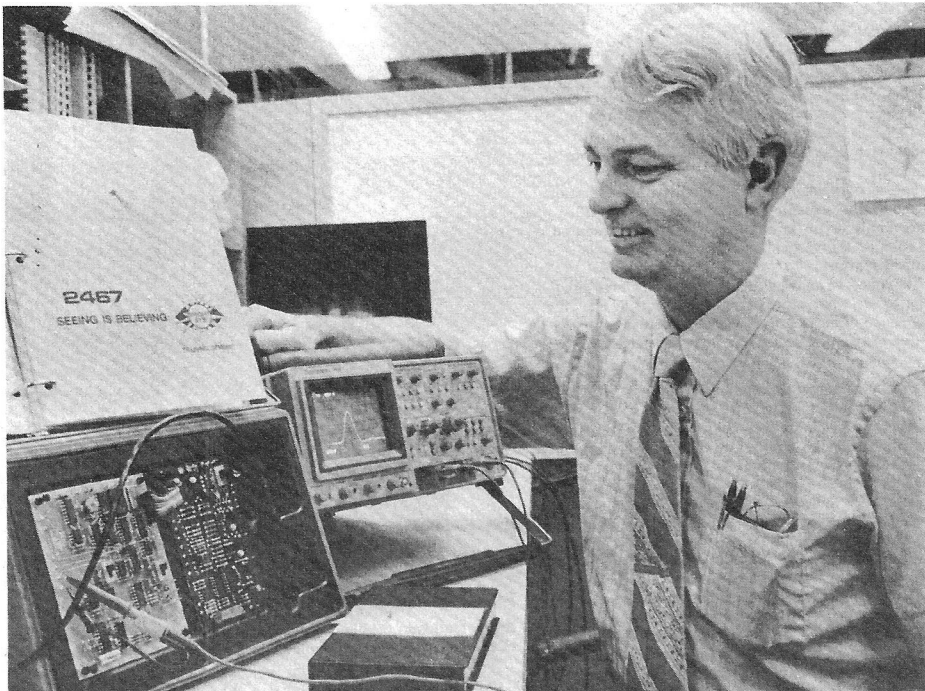
Rod Bristol says the 2467 portable scope—an analog instrument—will be a useful tool for designing and testing digital systems. Rod was one of the key engineers for the 2465 and is considered the prime advocate for adding microchannel plate technology to the 2465 "box"—a concept that is the basis for the 2467. The photo includes a demo kit and training package that sales engineers can share with customers.
