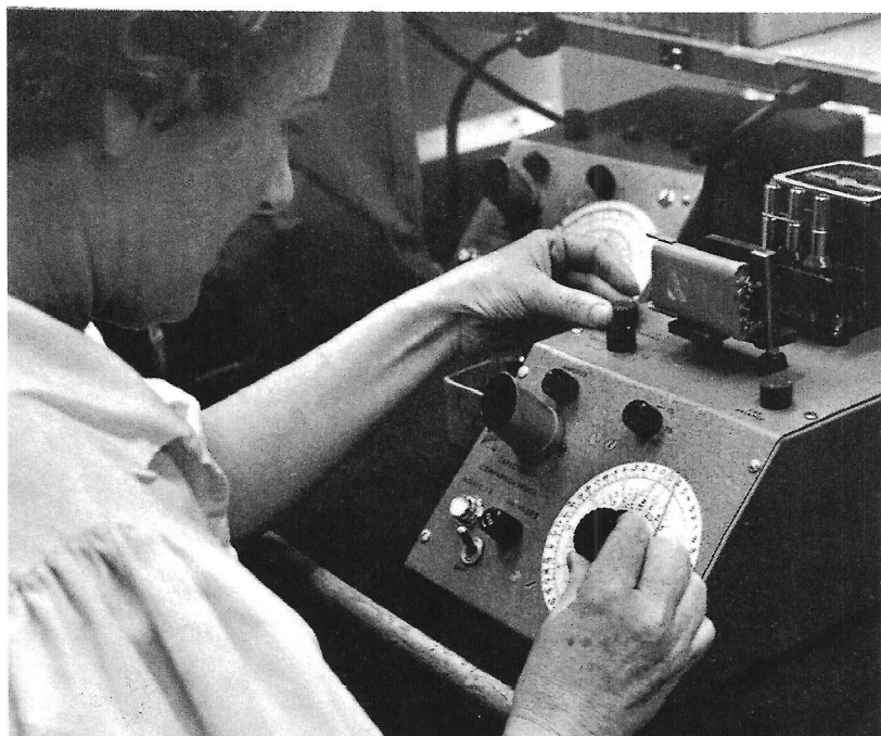
FINAL CALIBRATION OF TIMING CAPACITORS —The long-term accuracy of calibrated sweeps in Tektronix Oscilloscopes is due mainly to the extra emphasis we place on critical details in the design and manufacture of our sweep-timing capacitors. Careful control over dielectric absorption, leakage resistance, and impregnation help insure sweep linearity, timing accuracy, and general oscilloscope reliability.
