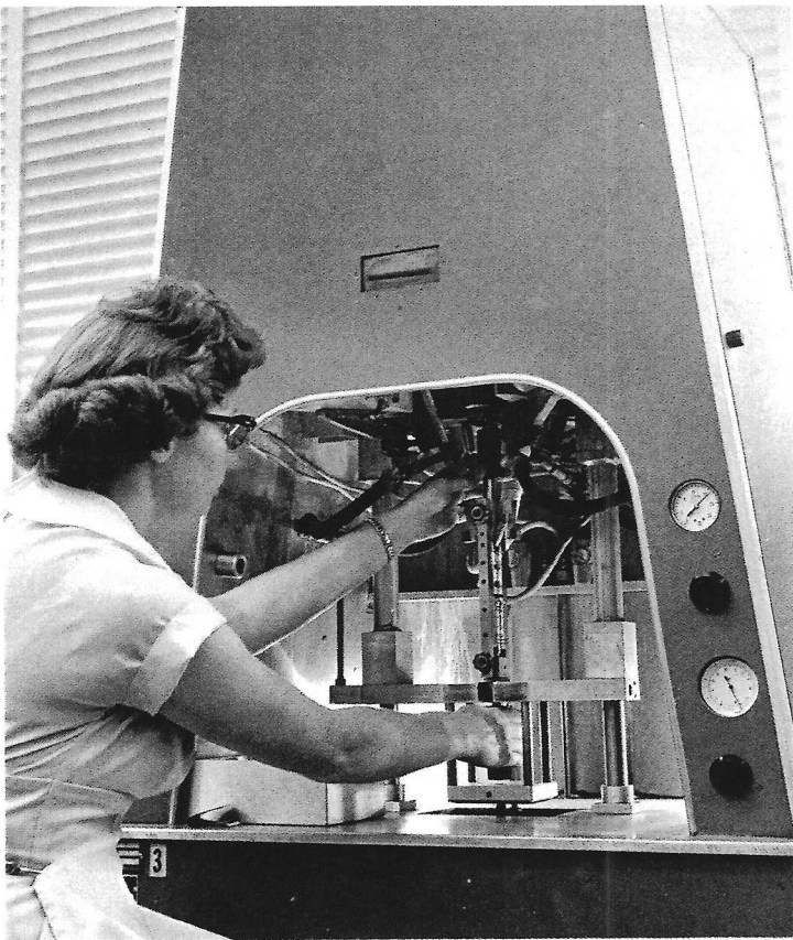
AUTOMATIC RODDING STATION —The glass rods that support electron gun assemblies of Tektronix cathode-ray tubes are applied in one operation to preserve the high alignment accuracy provided by precision jigs. Twenty-nine separate parts and assemblies make up the electron gun of the T555 dual-beam CRT, of which two, the vertical-deflection-plate assemblies, each contain fourteen separate parts.
