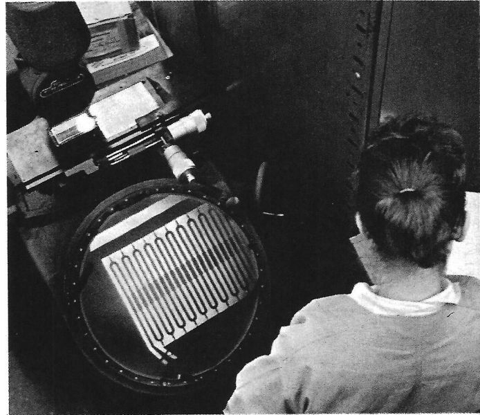
ACCURACY CHECK WITH OPTICAL COMPARATOR —The T519 cathode-ray tube, heart of the Type 519 dc-to-1 gc Oscilloscope, requires exacting manufacturing procedures. In this step the stripline of the distributed vertical-deflection system is checked with a magnifying optical comparator to an accuracy of \pm 0.0007 ". Material composition and temper, and thickness of plating are also very critical in this 3 mil-thick, 2\frac{3}{4} "-long cathode-ray tube part.
