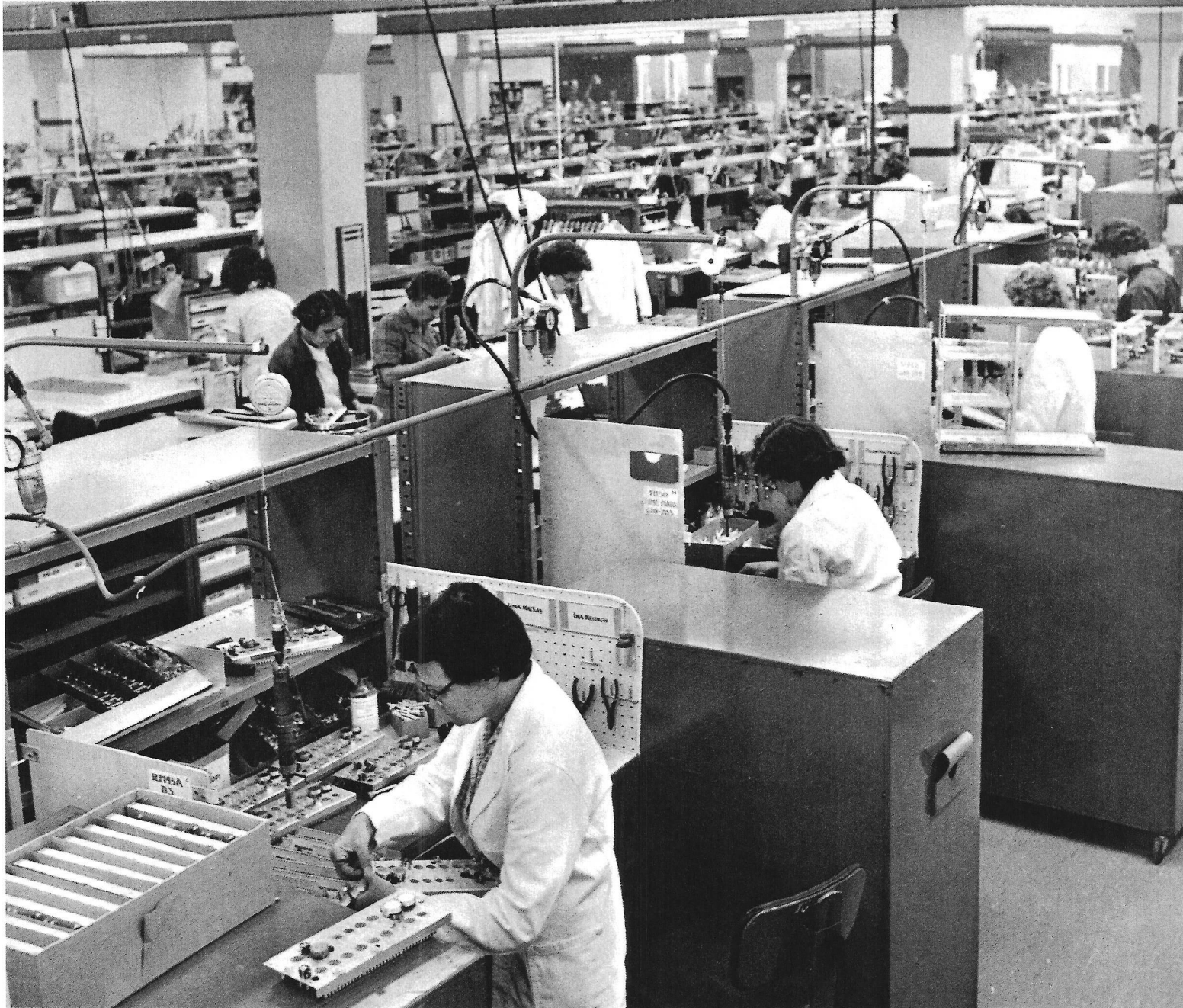
INSTRUMENT ASSEMBLY AREA —This is one of three large assembly areas located in buildings especially designed for this purpose. The assembler performs the complete mechanical assembly, and the wirer does all the wiring on each chassis or subassembly. The final assembler combines these with front and rear panels and structural members to form a complete instrument. The worker's responsibility for the complete job in his or her area fosters a strong feeling of pride in workmanship.
