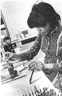
IRENE MANLOV is using a solder pot to solder coil wire ends to coil form leads, a quick process that tins the whole lead at the same time.
