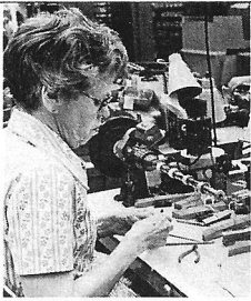
ROSE ROHRBACK, hand-winds high-voltage transformers, using very fine wire and delicate machinery. These components are much smaller than the low voltage power transformers shown in the last few pictures, and require different techniques and processes.
