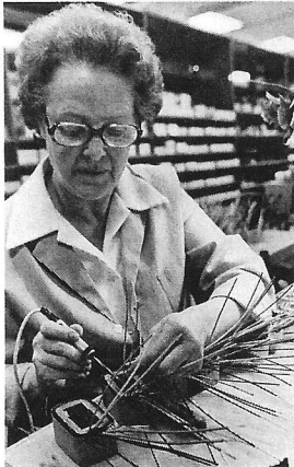
IN COIL FINISH area, Pat Gratreks (above) solders leads to ends of wires left extending from layers of insulation during winding; operator sometimes has to carefully probe between the layers to locate all the ends that have to be finished. In right photo, Mike Phonthany installs insulation sleeving over exposed wires left protruding in winding process; these will be self-leaded coils.
