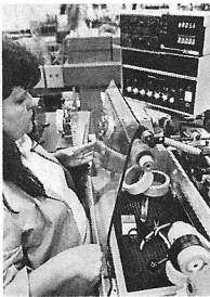
HOW DO YOU KNOW when you've wound the exact number of coils required? Jane Childers shows how it's done, with an electronic counter hooked up to winding machine.
