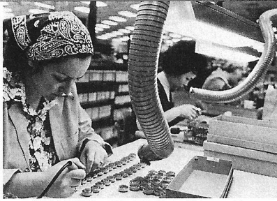
PAULA DOYLE and Judy Ro Kyung Kim are soldering tiny leads to the wires on these transformers, very delicate and precise work. Twisted tentacles of tubing in front of work benches are vents for carrying away solder flux fumes.
