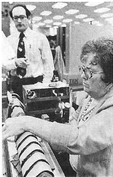
MARIE HAGGARD applies paper insulation to separate primary coils from secondary layers that will be applied in a later step. Each layer must be snug enough to stay firmly in place, but not tight enough to compress the layers.
