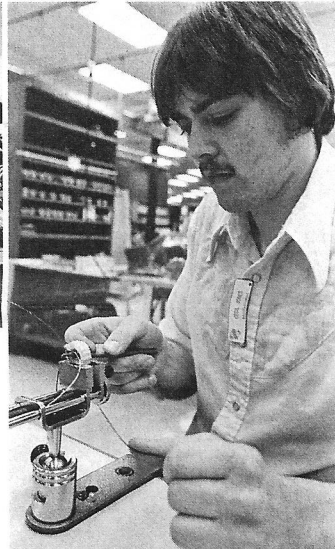
IS THAT REALLY a crochet hook? Yes, and it's the best tool we've found for hand-winding very heavy wire on a toroid coil. (We don't make enough of this kind to justify machinery investment.) Cecil Jones is making very precise windings by hand.
