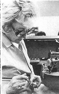
VERA NEFF machine-winds another kind of toroid coil, this one used for CRT deflection. At nearby bench, someone winding another kind of coil remarked, "This one is for the medical monitor." Tek people take a lot of interest in the finished products they're helping produce.
