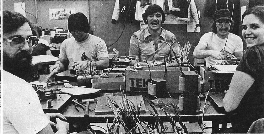
TRANSFORMER ASSEMBLY TEAM, left to right, Chuck White, Dave Tengan, Lee Oakley, John Bearden and Sandy Sherwood are performing "finish core insertion." Cores, thin pieces of metal, are inserted by machine into center of donut-shaped coil; then final pieces must be added by hand when core becomes too tightly packed for machine to finish.
