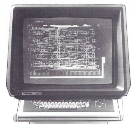
Tektronix plug-in intelligence options can be used with the 4016-1. Add-on low cost options include up to 26K of usable graphics display memory, scaling, relative graphics, clipping, circular arc generation, rotation by 1° increments, user definable stroke characters, programmable keyboard, GPIB interfacing to the intelligent 4924 Digital Cartridge Tape Drive, 4907 File Manager, and 4662 Interactive Digital Plotter, and local control of these peripherals plus the 4953 or 4954 Graphics Tablet.
