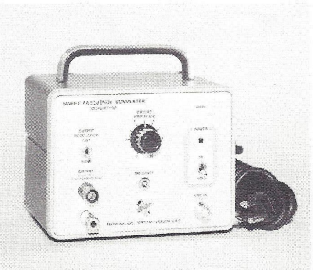
Swept frequency converter is designed as an accessory unit to the 1L5 and 3L5 plug-in units.
