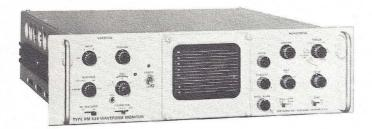
A new video waveform monitor, Type RM529 features extensive use of semiconductors—for new performance capabilities combined with high reliability. Low power consumption of 80 watts eliminates the need for a fan, insuring cool, clean, quiet operation.
