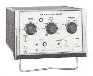
A new wide-range, general-purpose pulse generator, Type 114 features continuously-variable amplitude, pulse width, and pulse period. Pulse Risetime and Falltime is 10 nsec or less. Amplitude Range is 1 to 10 volts, positive or negative polarity, into a 50-ohm load impedance.
