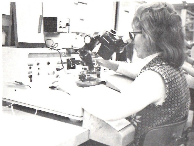
GOLD BONDING of IC's is a very exacting task, requiring the use of high powered microscopes. Nancy Anderson is the operator.
