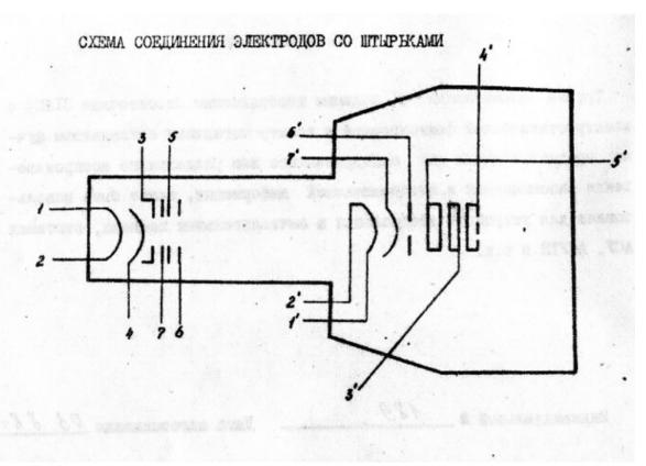
Connection diagram of electrodes with pins
