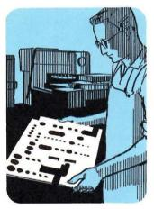
A chassis panel is removed from the press, having been punched out to its exact pattern without help from the operator.
