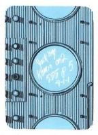
Performance data and date checked are recorded right on the CRT face. This life expectancy test is one of the most revealing in Tektronix' quality assurance program.
