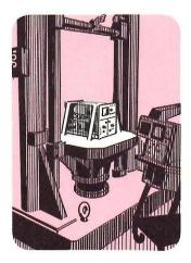
Shock forces measured in scores of G's are applied to Tektronix oscilloscopes on this drop-test apparatus weighing several tons. The shock wave is recorded on another storage oscilloscope.
