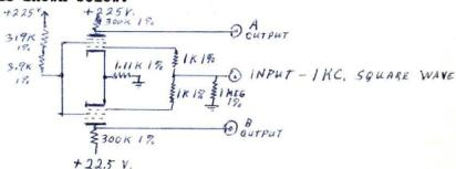
A 100 MV k LC square wave signal is fed to the grids of the two tubes being paired. Output from these tubes as observed on a scope must not exceed .34 volts peak-to-peak to be an acceptable pair.
