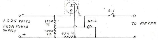
When complete, the assembly is plugged into checker. If neon lights, there is an error in assembly. If neon does not light, press switch (s-1). Meter should read between 10 and 40 volts.
