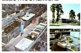
Electrochemical laboratories, engineering support, and a large production capability provide many special parts for today's oscilloscopes. Chemical machining can quickly produce prototype parts for evaluation by design engineers while maintaining critical tolerances. Precision electroplating of plastics and other materials, and electroforming intricately shaped parts are daily tasks of our electrochemical department.
