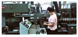
Plastics technology provides Tektronix with many components. Voltage and current probe parts are made with special plastics that reduce undesirable electrical effects and withstand rugged use. A special packaging material protects instruments and parts during shipment. Other plastic parts include special switch couplings, handles, knobs, capacitor mounts and covers, and many other items designed to optimize oscilloscope performance.
