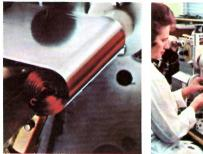
Timing capacitors and input-coupling capacitors are critical components in oscilloscope performance. Building our own capacitors permits us to meet specific performance requirements and make special sizes and mounting configurations.
