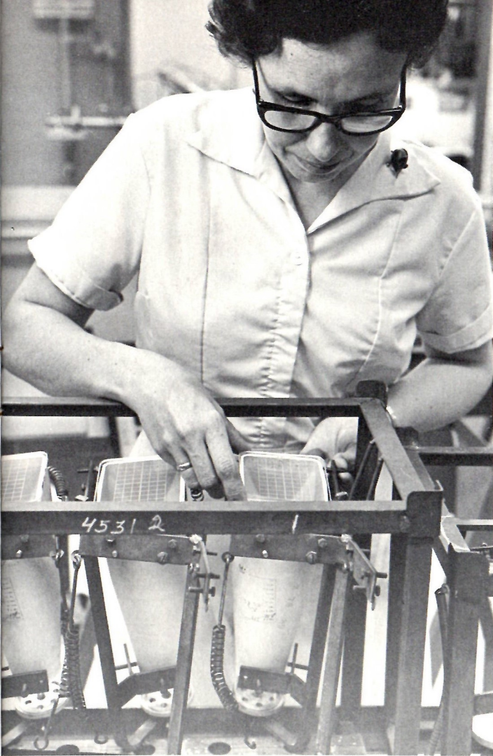
MELTING OF GLASS pre-form (opposite page) around funnel's metal pin is shown in this neck-pin beading operation. Funnels are held in jig (top left) during faceplate-seal firing, and weldings on gun assembly are inspected after stem attachments (top right). CRT targets (bottom) are inspected and covered by plastic faceplates prior to "potting."
