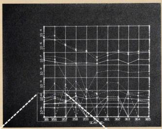
DISPLAY SCALE—selects display size and provides vertical and horizontal magnification. Aspect ratios are selectable from 32:1 to 1:32. To magnify, a scale size is selected; a scaled "Frame" is positioned to window a portion of the plot. When replayed, the "Framed" portion of the plot is replotted as a full screen display.
