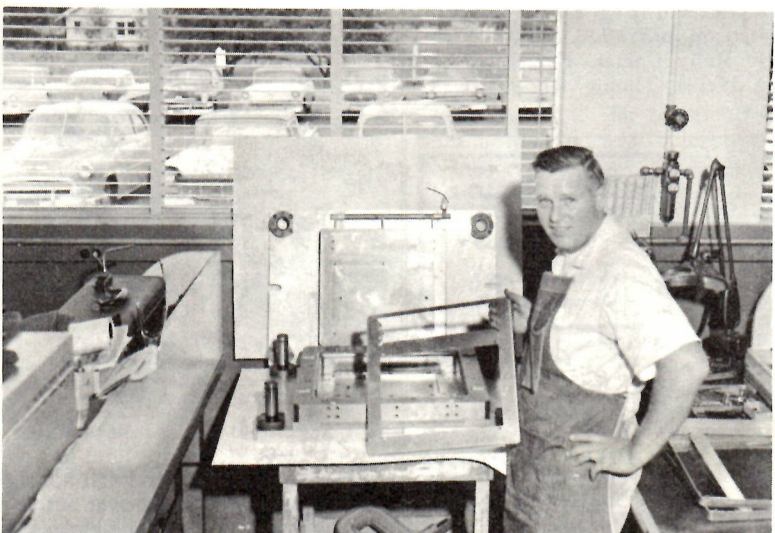
An example of the product of the Production Tooling department is this Draw Die for the new Scopemobile front panel. With this type of precision tooling the Shop is equipped to meet the demands of Production.
