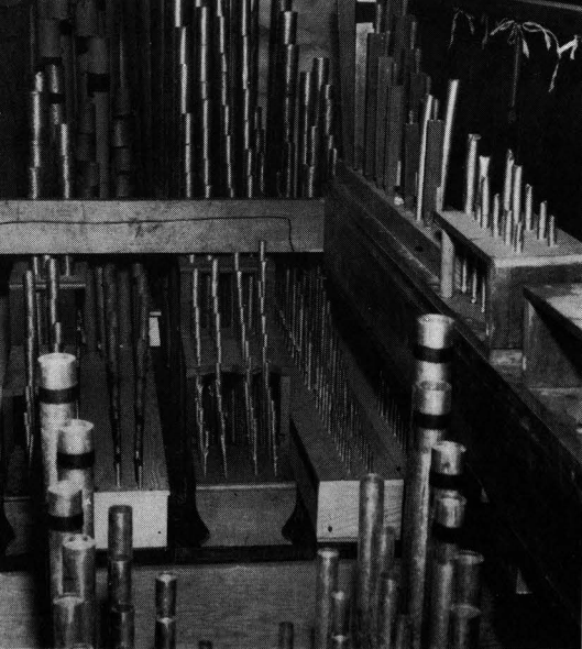
Principal/Percussion chamber showing Diapason chorus with mixture in foreground and independent 2-2/3' Flute at extreme right. Note cone tuning.
