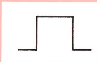
**Fig. 12. Illustrating accentuated high-frequency response as a result of probe misadjustment.**
