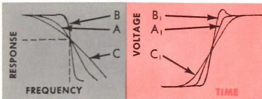
**Fig. 16. Effects of high-frequency compensation on square waves.**
