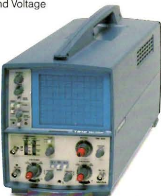
T912 Bistable Storage • 250 div/ms Stored Writing Speed. (1 cm/div CRT) • DC-10 MHz • 2 mV/div Vertical Sensitivity • Dual trace • Delay Line
