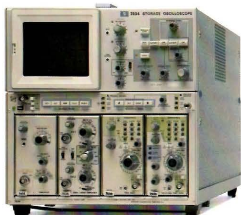
7834 Basic System Multimode Storage Bistable, Variable Persistence, Fast Transfer • 5500 div/μs Stored Writing Speed (reduced scan—45 cm/div) • 300 div/μs Stored Writing Speed (0.9 cm/div CRT) • DC-400 MHz Bandwidth • 3 Vertical Channels • Delta time CRT Readout
