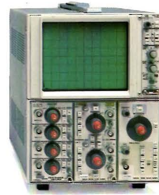
5113 Basic System Split Screen Bistable Storage • 20 div/ms Stored Writing Speed (1.27 cm/div CRT) • 200 div/ms with Opt 03 • DC-2 MHz Bandwidth • Dual Beam • Six Vertical Channels
