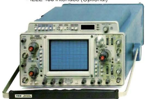
468 Digital Storage • 10 MHz Useful Storage Bandwidth • 100 MHz Non-Storage Bandwidth • Cursors for Time and Voltage Measurements • Envelope Mode • Signal Averaging and IEEE 488 Interface Options
