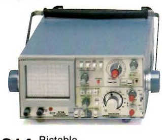
314 Bistable Storage • 400 div/ms Stored Writing Speed. (0.6 cm/div CRT) • DC-10 MHz Bandwidth • 1 mV/div Vertical sensitivity • Dual trace • Lightweight ≈10.5 lbs.
