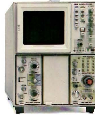
7613 Basic System Variable Persistence Storage • 5 div/μs Stored Writing Speed (0.9 cm/div CRT) • DC-75 MHz • 5 mV/div Vertical sensitivity • Dual Trace • CRT Readout
