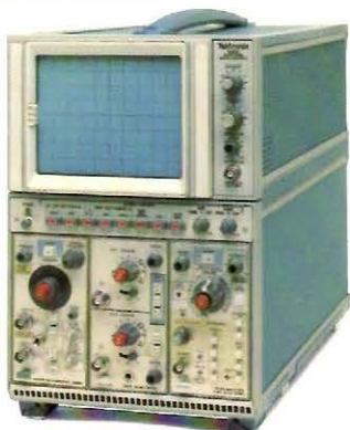
5223 Digital Storage (with 5B25N) • Stores Repetitive Waveforms up to 10 MHz • Pretrigger • Roll Mode • X-Y Plotter Output with Penlift • IEEE 488 Interface (Optional)
