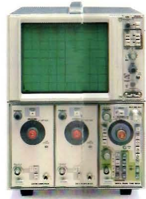
5115 Basic System Split Screen Bistable Storage • 800 div/ms Stored Writing Speed (1.27 cm/div CRT) • DC-2 MHz Mainframe • 1 mV/div Vertical sensitivity • Dual trace • Dual time base
