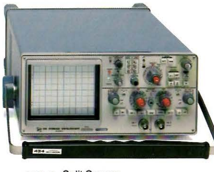
434 Split Screen Bistable Storage • 400 div/ms Stored Writing Speed. (0.97 cm/div CRT) • 5000 div/ms with Option 1 • DC-25 MHz Bandwidth • Dual trace • Wide Range Magnifier
