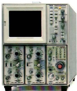
7633 Basic System Multimode Storage Bistable, Variable Persistence, Fast Transfer • 2200 div/μs Stored Writing Speed (reduced scan—45 cm/div) • 150 div/μs Stored Writing Speed (0.9 cm/div CRT) • DC-100 MHz Bandwidth • 5 mV/div Vertical sensitivity • Dual trace • CRT Readout
