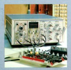
And, if you're keeping a close measure on costs, remember that a significant part of the price of every single-function instrument is its power supply. But with TM 500, one power supply is shared by several instruments, so you can add on more performance capabilities for less money.
