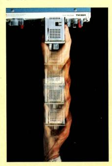
Several words came close to describing this idea. One was modularity. Each TM 500 device—whether a multi-meter or power supply, oscilloscope or logic analyzer—is designed as a plug-in module to fit into any TM 500 mainframe with other modules. Instruments are interchangeable in seconds so you can slip together a system for one test, then rematch the set using other modules for a completely different application. Nearly 40 different TM 500 instruments are available.
