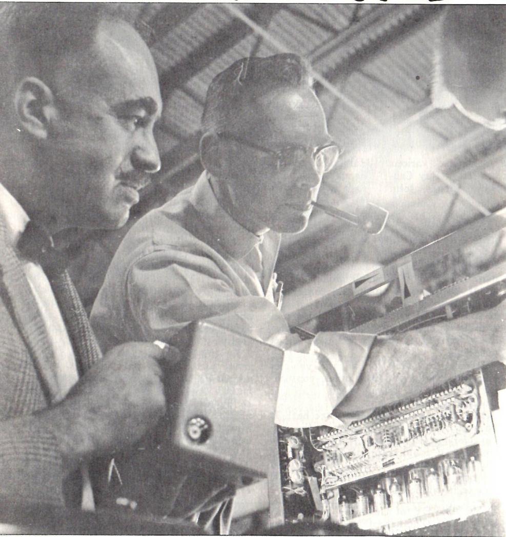
FRANK MANIATIS (left) and Bob Poulin watch intently as a 945 militarized scope is shaken violently on a vibration table, part of the torture treatment which is our environmental testing program. They're using a repeating strobelight to "slow down" the scope motion, which otherwise would be too fast for the eye to observe.
