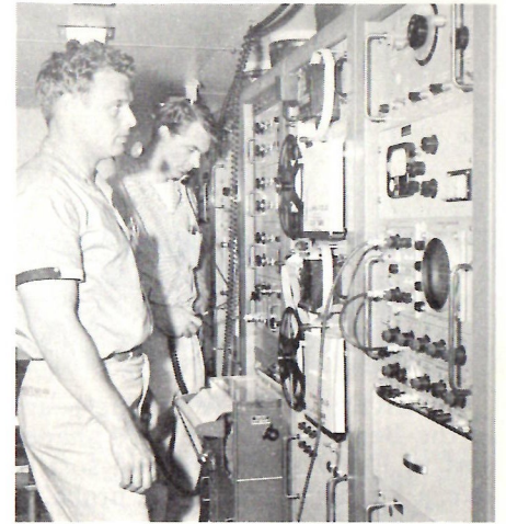
FRITZ VON Pilgrim (foreground) and Wayne Holm of Space Technology Laboratories, Los Angeles, check out guidance equipment for tracking the Explorer Paddlewheel satellite. Prominent is a Tek rack-mounted scope.
