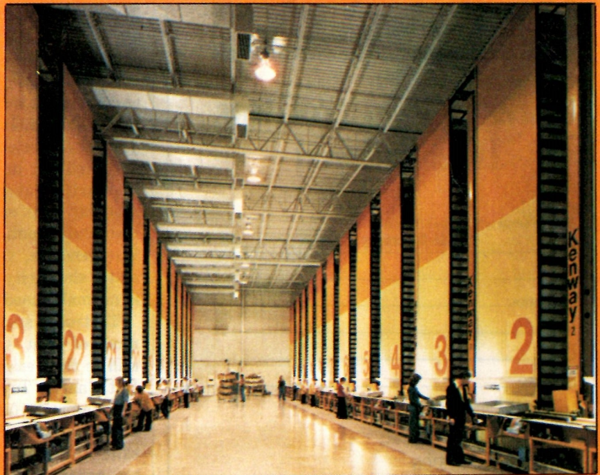
Approximately 65 percent of the 130,000-part lines stored in the automated Tektronix warehouse are housed in the miniload section. Two DEC PDP 11/70 computers keep track of where each part is in the storage process.
