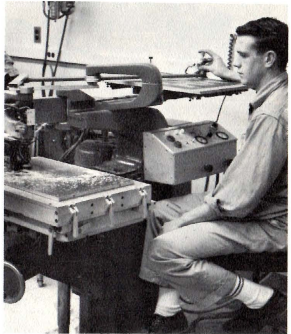
CHEMICAL PROCESSING FLOOR of new building holds all plating and anodizing tanks (upper left). Network of special resin-treated plumbing and ventilation pipes interlace under the chemical process area grids (lower left). Machine operator reproduces 24 panels at one time, using pantograph (right).
