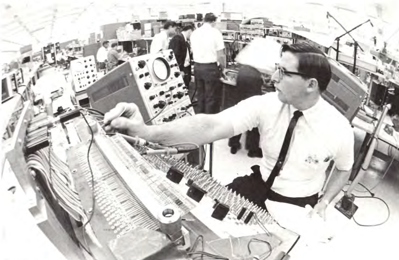
COMPUTER ELEMENTS for US Air Force's C5A jet transport are checked out at Northrup Corporation. Tektronix oscilloscopes are among the test instruments.
