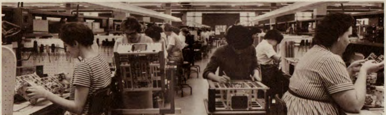
TEKTRONIX' LARGEST operation is Instrument Assembly. Here, skilled employees assemble and wire the intricate oscilloscope chassis.
