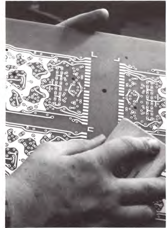
ETCHED CIRCUIT boards are among the components manufactured at Tektronix. In the 454, boards provide critical spacing and alignment, enabling instrument portability as well as high performance.
