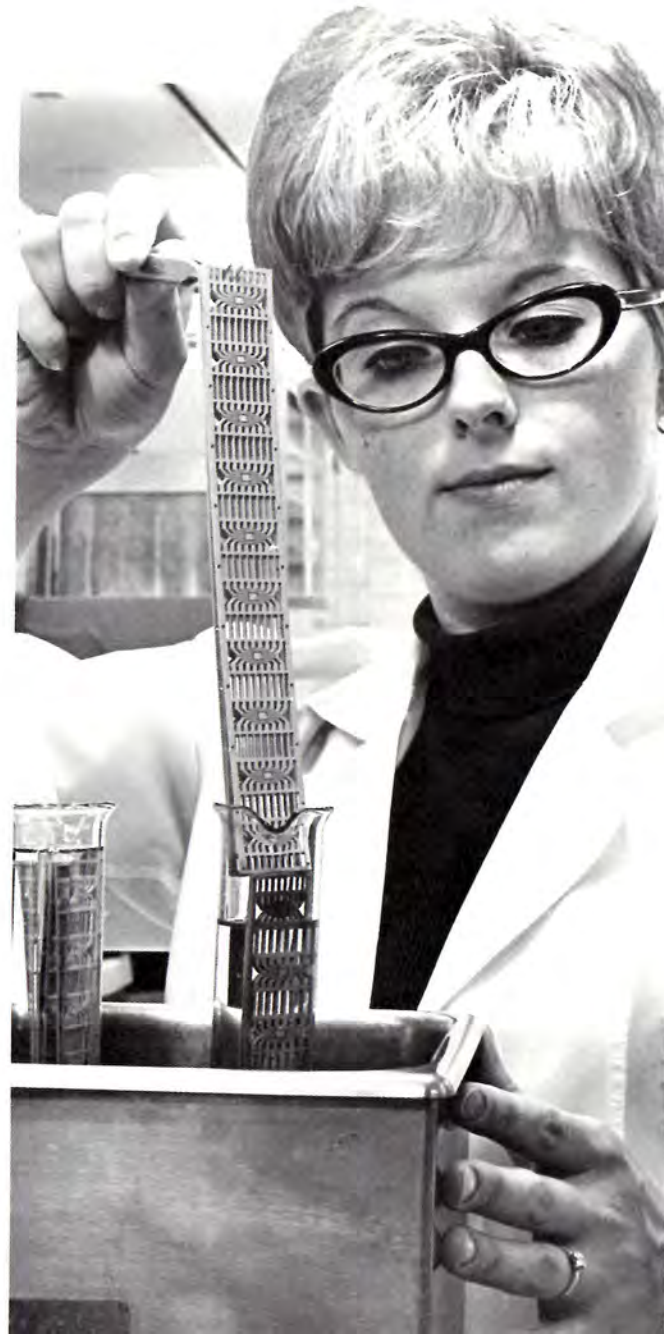
CLEANING OF dual in-lines is a critical step in the production of Tektronix special-purpose integrated circuits.
