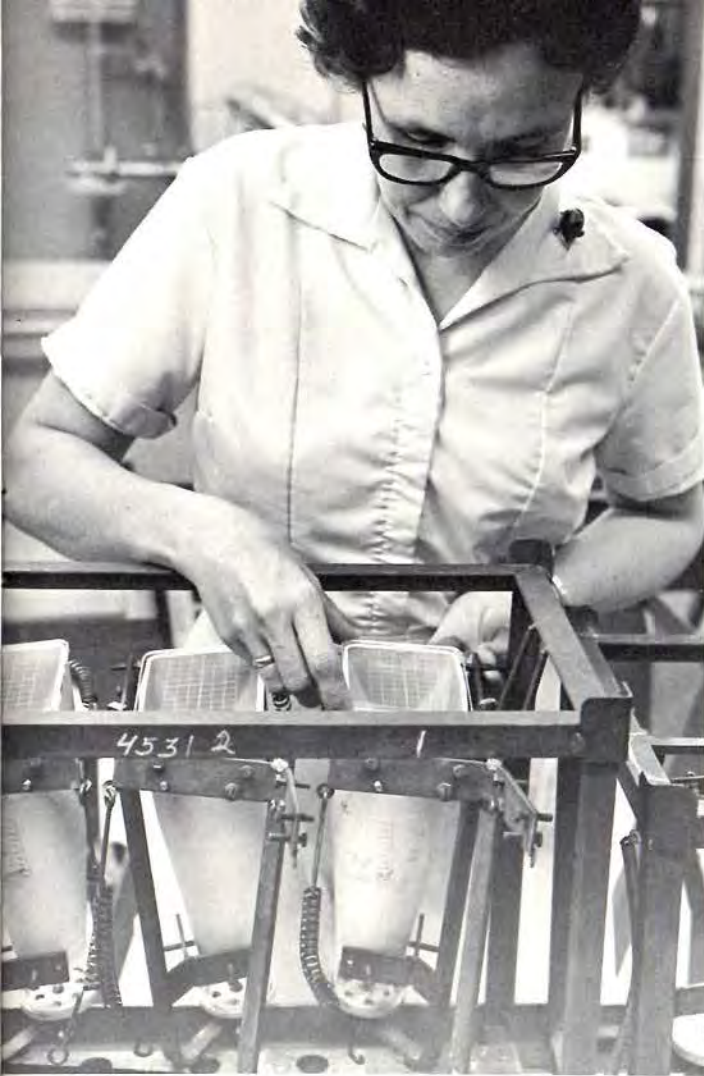
MELTING OF GLASS pre-form (opposite page) around funnel's metal pin is shown in this neck-pin beading operation. Funnels are held in jig (top left) during faceplate-seal firing, and weldings on gun assembly are inspected after stem attachments (top right). CRT targets (bottom) are inspected and covered by plastic faceplates prior to "potting."
