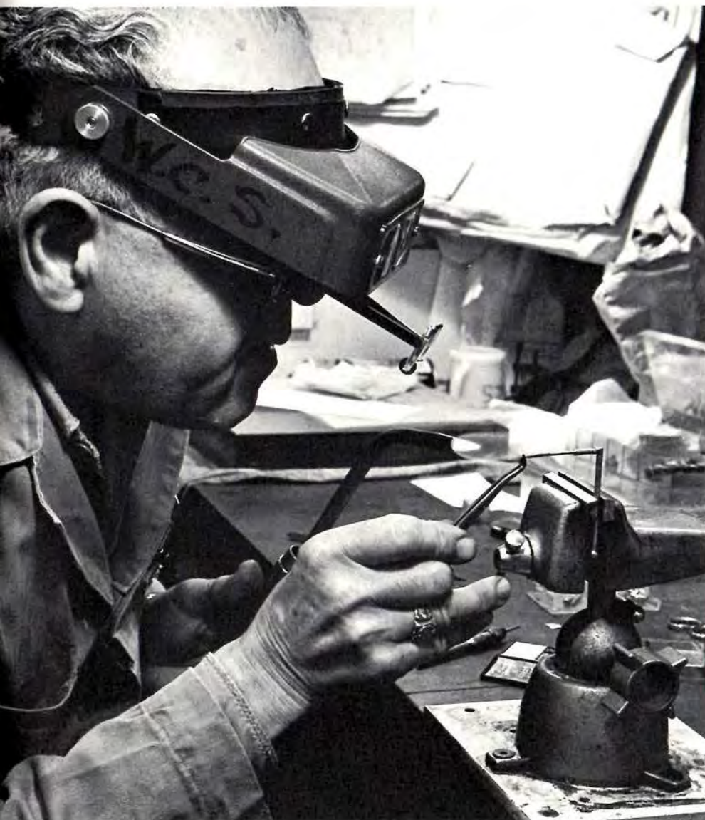
PRECISION NOZZLES (bottom photo) are fabricated for sand-blasting lines in metal-coated funnels. A "clean room" (top photo) is required for fabricating storage-type targets.
