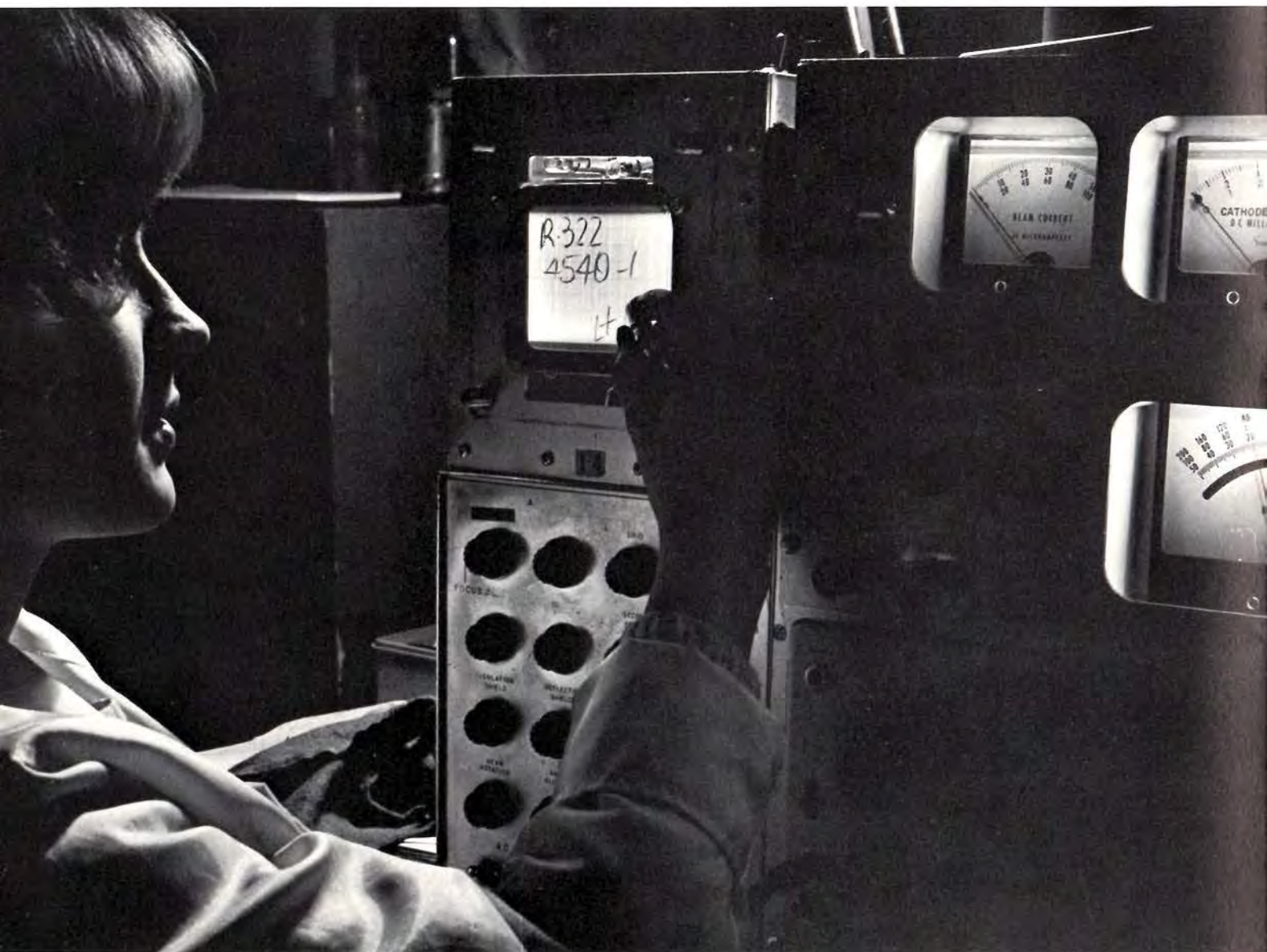
NUMEROUS ELECTRICAL measurements are made during final testing of ceramic CRTs.
