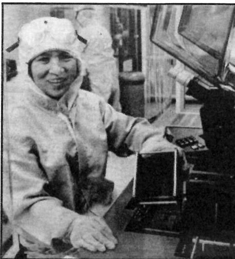
PHOTO TECHNICIAN Merlina Fagaragan loads CCD wafers into a projection aligner used for printing millions of tiny, precise patterns.
