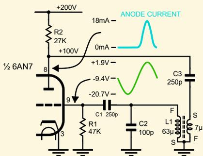
**Figure A: a typical AM radio oscillator configuration. The T-130’s implementation is shown at lower right in Figure D.**
