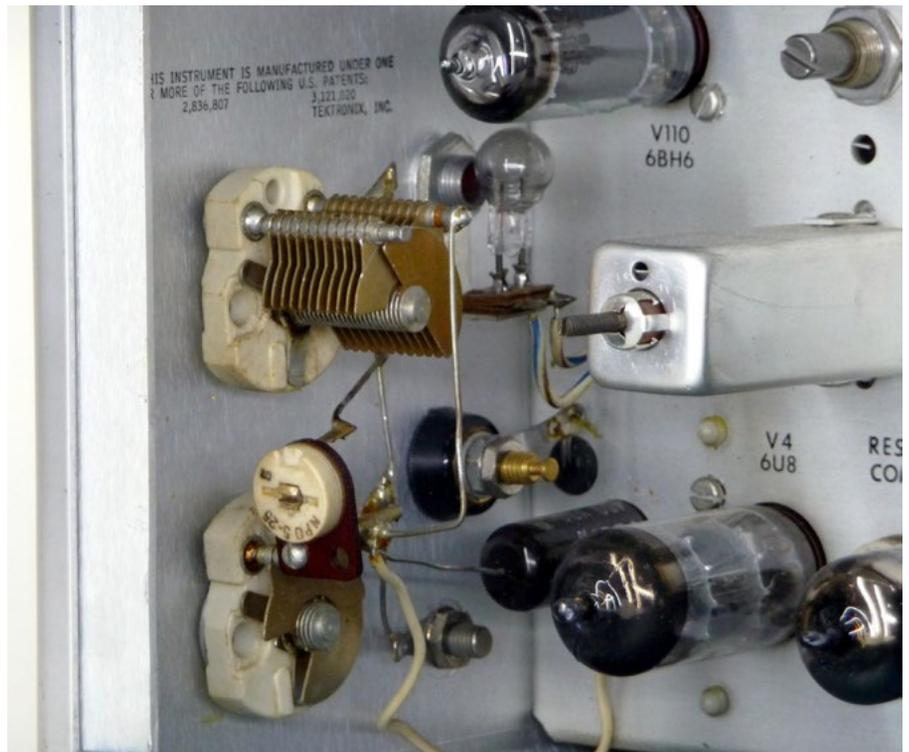
A close-up of part of the variable oscillator section, incorporating V4 and variable capacitors C2-C5, as described in the panel labelled "An ingenious oscillator design".
