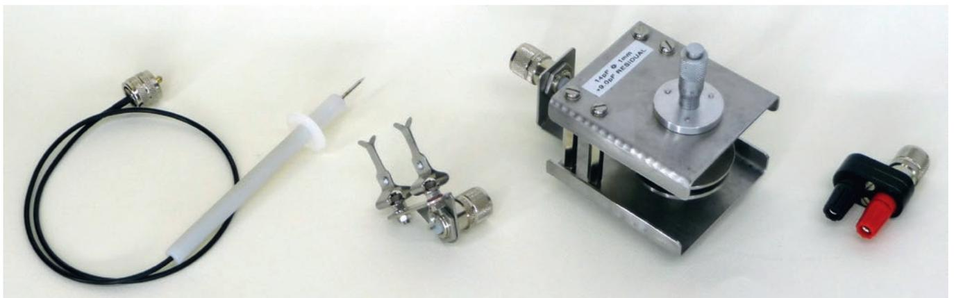
Shown above are a variety of homemade adaptors which can be connected to the UNKNOWN jack on the front panel. The largest one (second from the right) is a variable space capacitor for measuring permittivity – the degree that an insulating material increases capacitance between the plates over the capacitance obtained with air or vacuum spacing.
