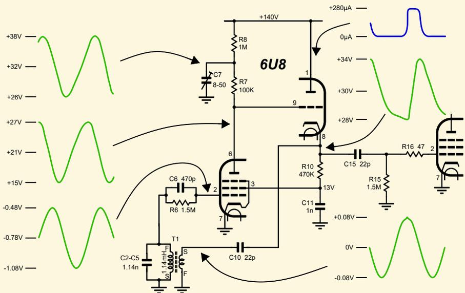
Figure D: the variable oscillator configuration used in the T-130 uses a 6U8 triode pentode.
