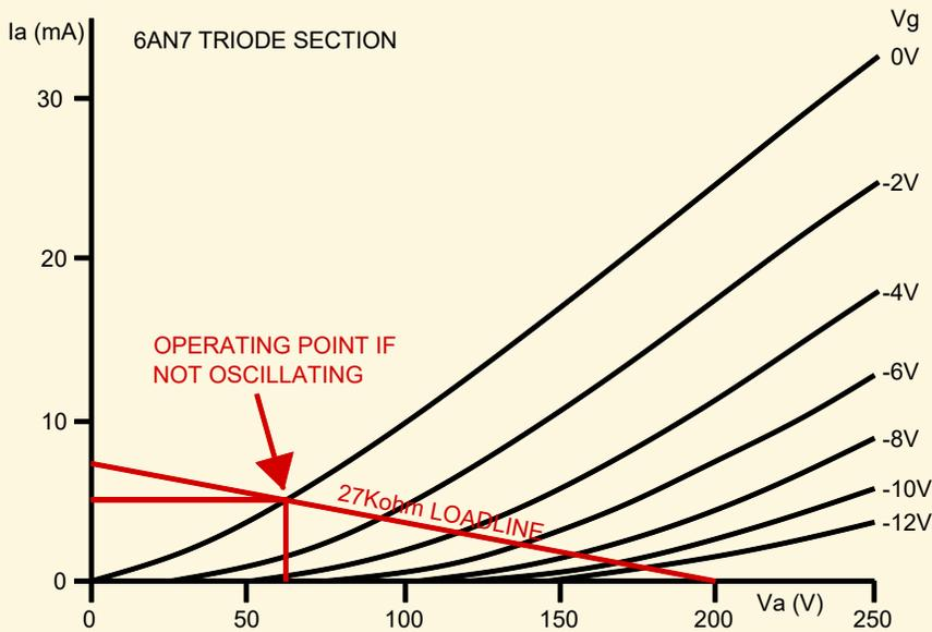
Figure C: plot of the 6AN7's anode voltage versus anode current for various grid bias amounts. The 27kΩ is the load connected to the plate of the 6AN7 (R2 in Figure A).
