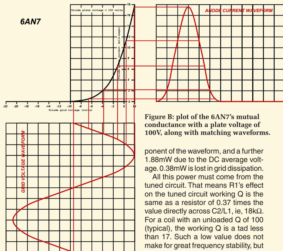
**Figure B: plot of the 6AN7’s mutual conductance with a plate voltage of 100V, along with matching waveforms.**
