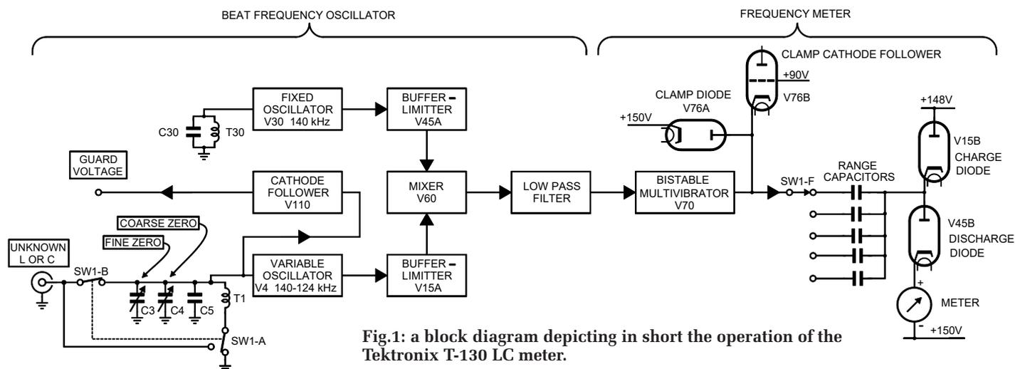
Fig.1: a block diagram depicting in short the operation of the Tektronix T-130 LC meter.
