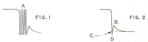
The TRIGGER SENSITIVITY control should now be gradually turned CCW until the self-oscillation indicated at A just dies out. The result is a display shown in the solid line of Fig. 2. The TRIGGER SENSITIVITY control should be turned further in the CCW direction until the peak B drops to a point C (dotted line, Fig. 2) which has a height above D equal to one-half its original height.
