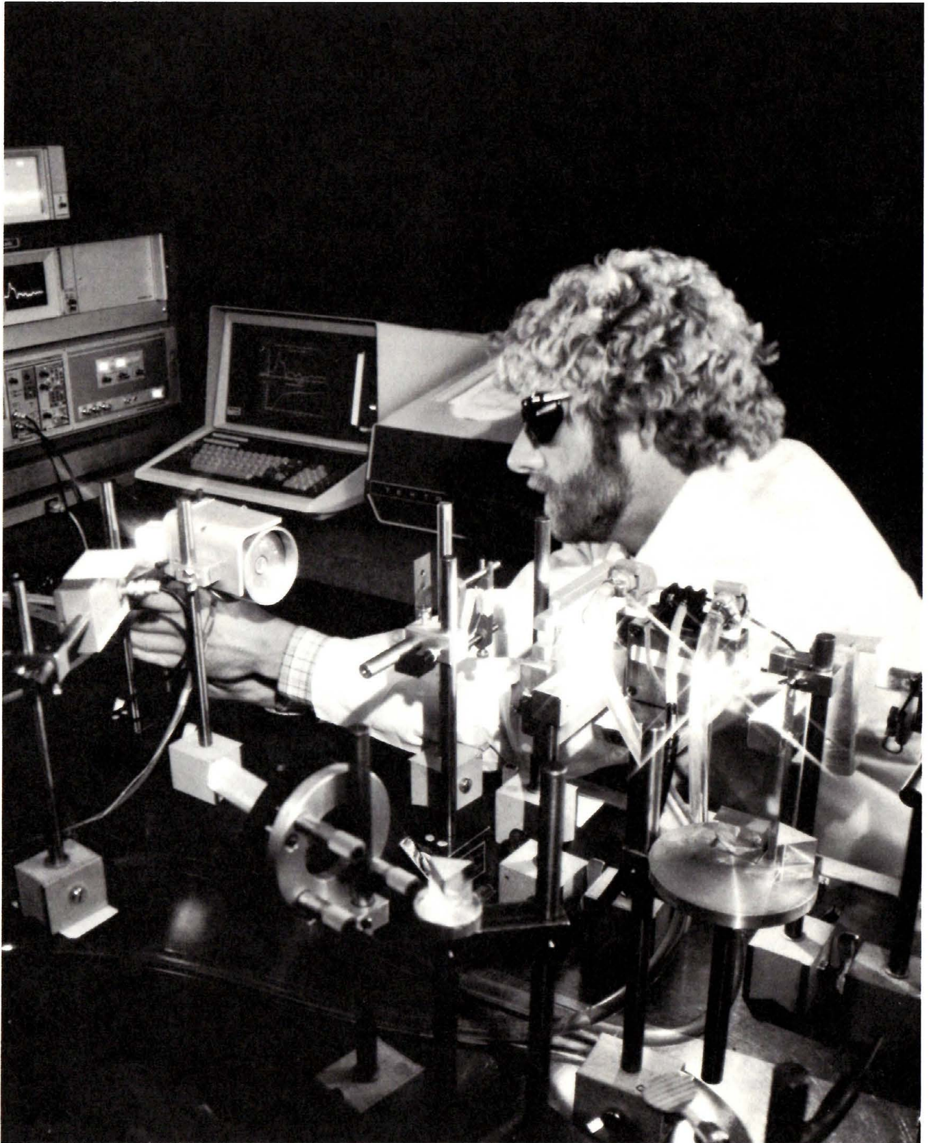
TEKTRONIX signal-processing system monitors a repetitively pulsed ND:YAG laser and frequency doubler, at Oregon Graduate Center for Study and Research.
