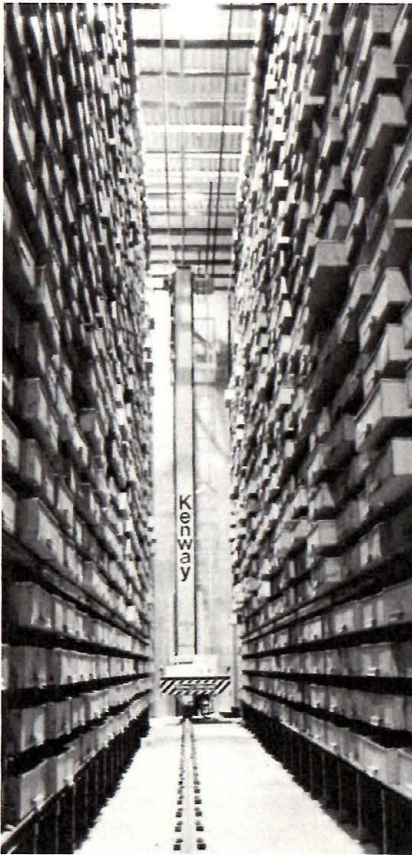
AUTOMATED CRANES serve small-parts storage area in new warehouse.
