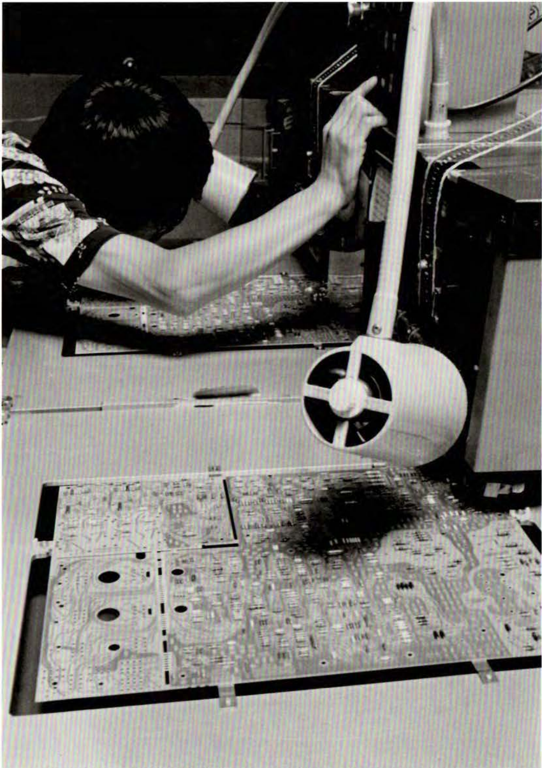
COMPONENTS ARE machine-inserted into printed circuit boards, as part of the production of 2200-series oscilloscopes.
