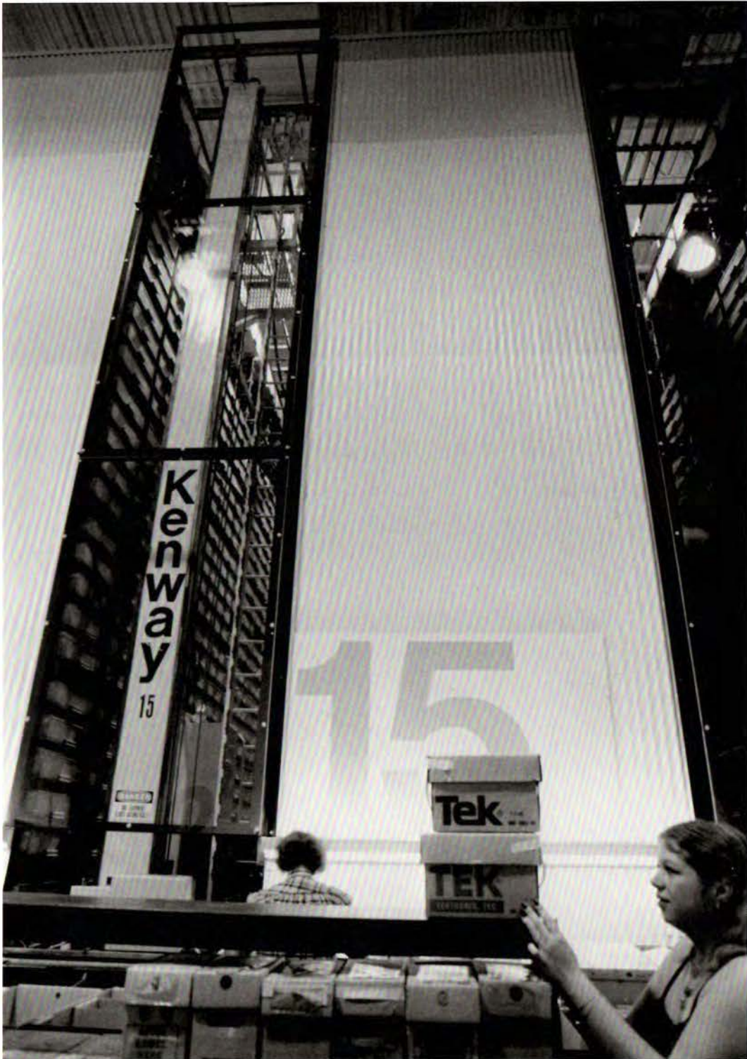
NEW AUTOMATED WAREHOUSE, which went on-line this year, enables computer management of parts and materials.
