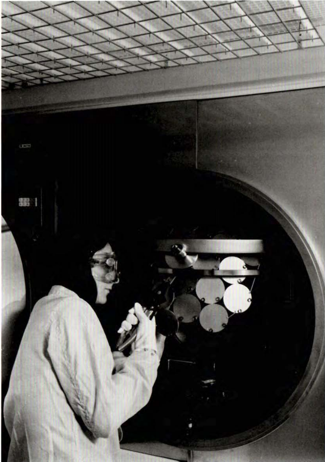
TECHNICIAN REMOVES a wafer platen after an aluminum coating has been deposited on integrated-circuit wafers.
