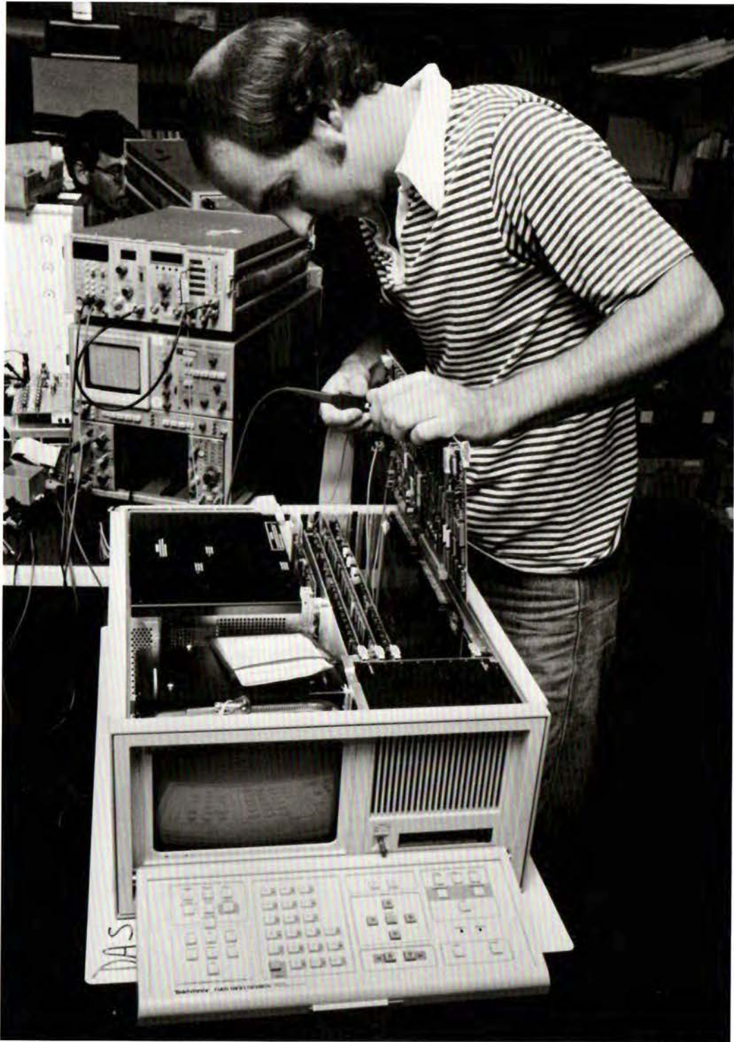
NEW DAS 9100 SERIES digital-analysis system undergoes test operation. Plug-in circuit boards adapt mainframe to a variety of digital-analysis tasks.
