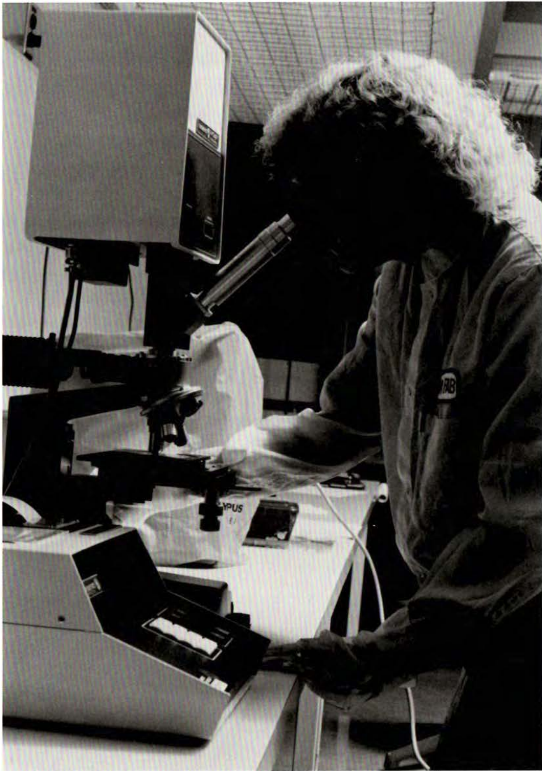
INSPECTIONS ARE FREQUENT during the production of integrated circuits. Here, wafers undergo one of many visual checks that insure top-quality products.
