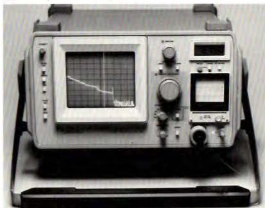
OF150 measures signal losses in optical cable.
