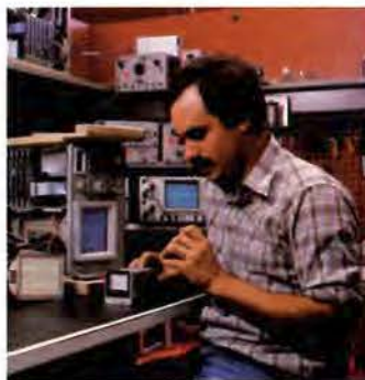
CHART RECORDER for OF150 fiber optic cable tester is calibrated.
