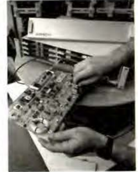
FIBER OPTIC cable is connected to this board. A laser diode sends light down the cable.
