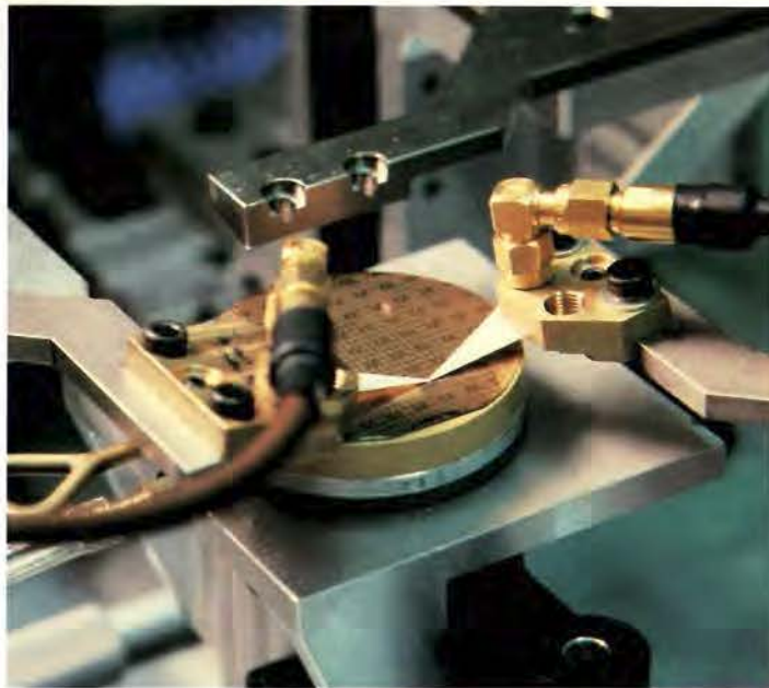
TEK-DEVELOPED high-frequency probe for ICs on wafers (above) enables measurements up to 18GHz, making it the fastest wafer probe in existence. (Close-up at left.)
