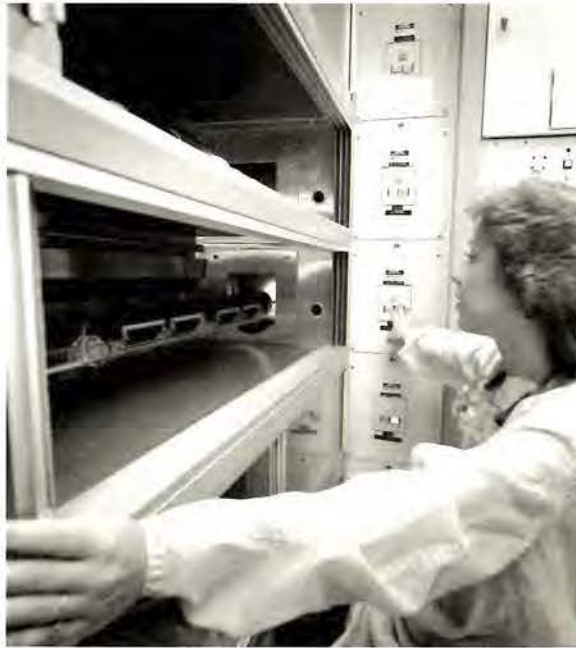
SILICON WAFERS in the oven during fabrication of integrated circuits.
