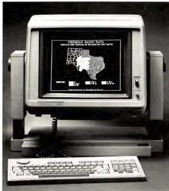
The 4105's versatile display stand tilts, swivels, glides and elevates to suit the user's preferences.
