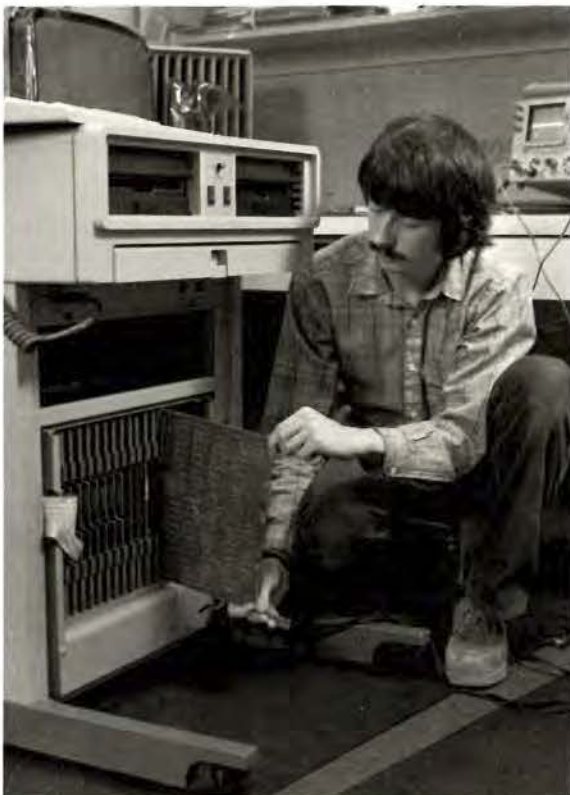
CIRCUIT BOARDS are inserted and tested in the pedestal of our 4115B color graphics terminal.
