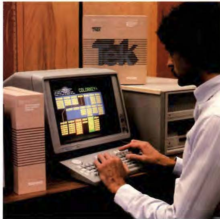
LANDS (Language Development System) is one of our most important software products. It is used here on a new Tek 4105 color terminal. Our color interface, ColorKey +™ is the only one offered by any microprocessor development system.
