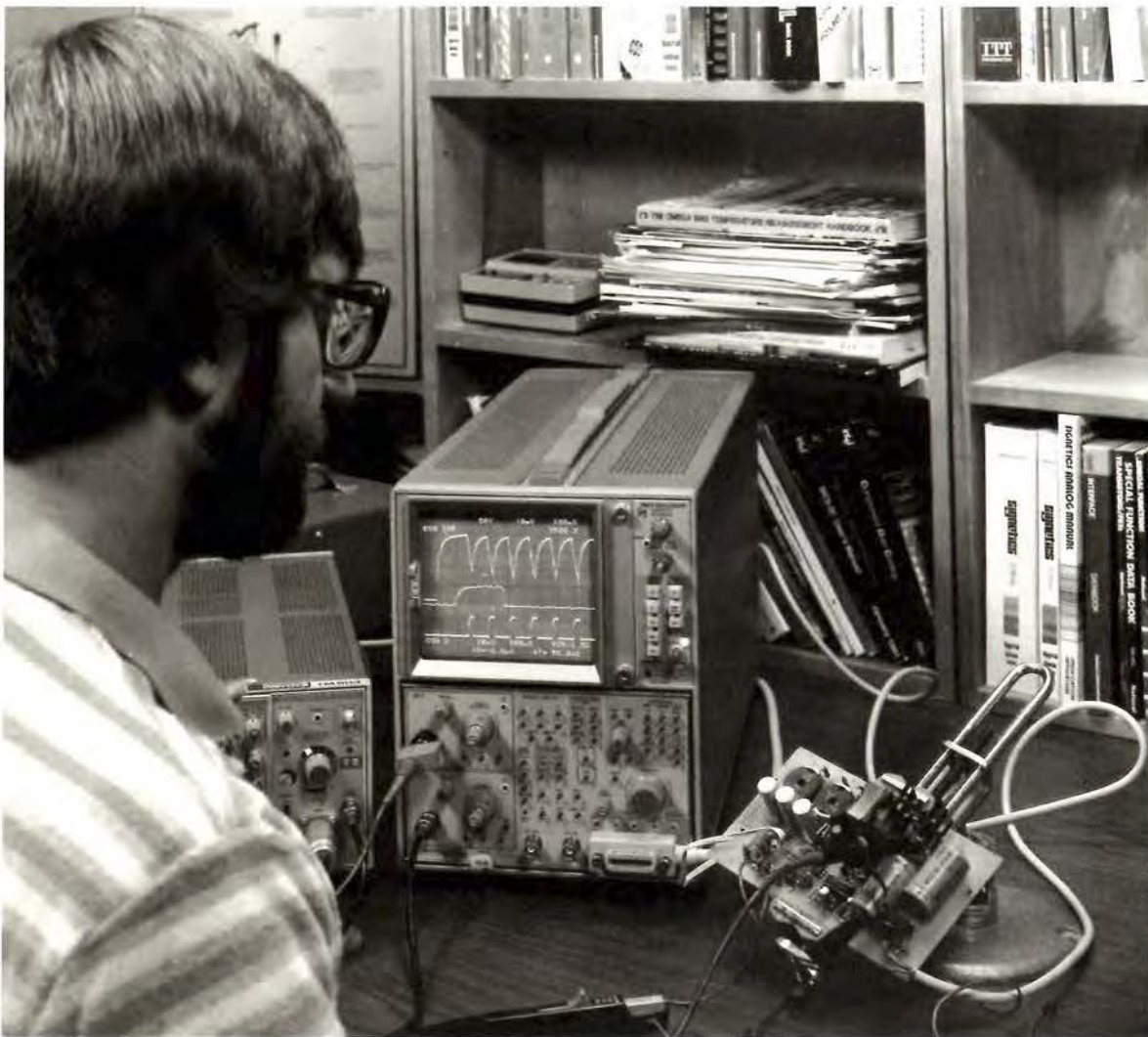
ANY TEK LABORATORY oscilloscope can now be instantly converted to digital use by inserting our new plug-ins. The 7D20, shown here, was designed for use with 7000-series lab scopes. Above, its "envelope" mode, setting the bounds for go/no-go tests, allows less-trained people to use the 7D20's capabilities.
