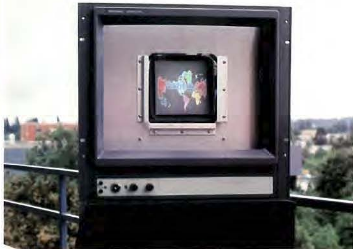
THE BRIGHT daylight would wash out most color displays, but the Tek T8100 CRT produces a highly visible image. It will be used at first in avionics.
