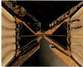
TEK-DEVELOPED high-frequency probe for ICs on wafers (above) enables measurements up to 18GHz, making it the fastest wafer probe in existence. (Close-up at left.)
