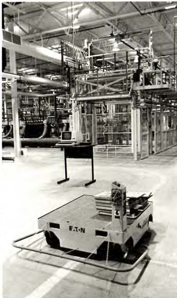
NOBODY IN THE picture at Forest Grove? That's the way it often is at our highly automated circuit-board plant. Here, an unmanned delivery cart responds to a computer command, guided by an electrical circuit in the floor. Below, circuit boards move along untouched by human hands.
