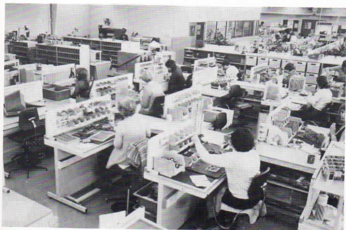
A part of the Production Area, mainly engaged on building the Telequipment D1000 series of oscilloscopes
