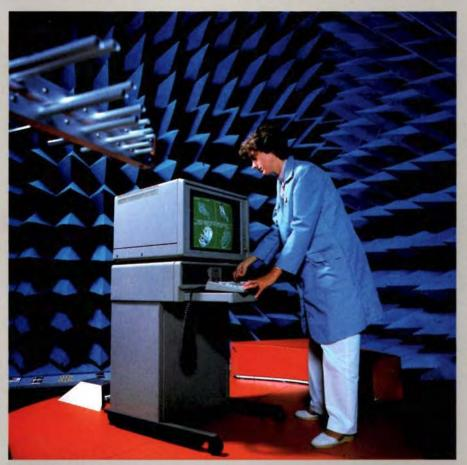
diagramming, and its "zoom" capabilities where parts of the screen are selectively enlarged. At the magnification of the zoomed section (lower right, inset), the full cathode ray tube screen would cover half a football field. To meet increasingly stringent international standards, the 4115B is tested for electromagnetic noise in an "anechoic chamber" (left) at Tek.
