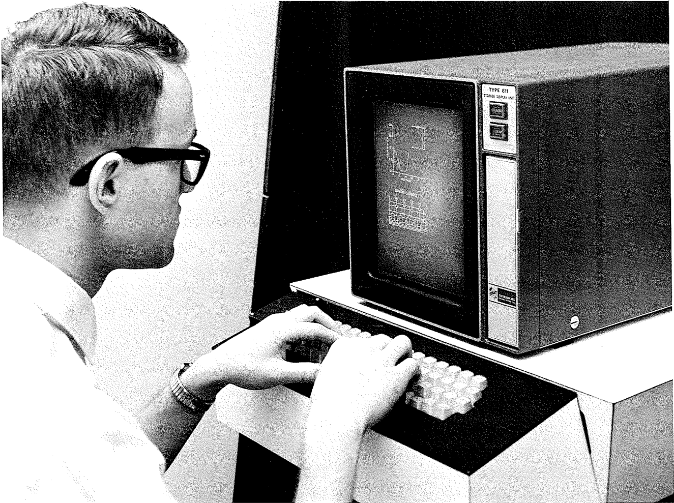
Ray Goolsbey, Tektronix Digital Instruments Engineer, checks out his programs on the Type 611 Storage Display Unit. See photo on page 9.
