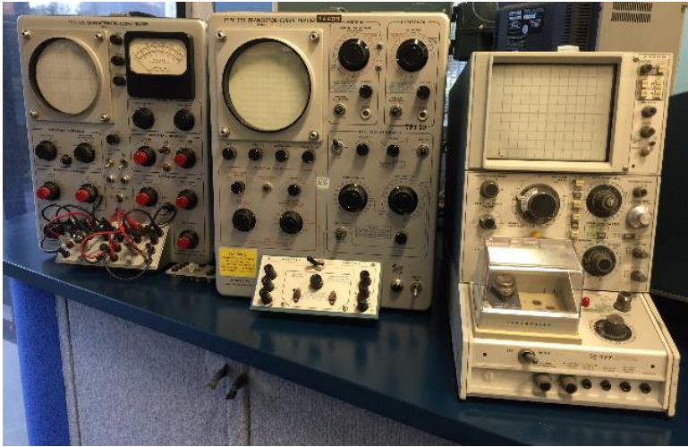
Here are three of the museum's curve tracers. L to R: Types 570, 575, 577
