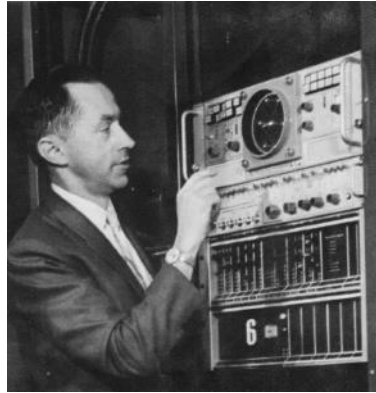
Charles Rhodes adjusting a Type 520 Vectorscope
