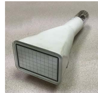
The CRTs used in the 200 series scopes were the smallest tubes Tek ever made.
