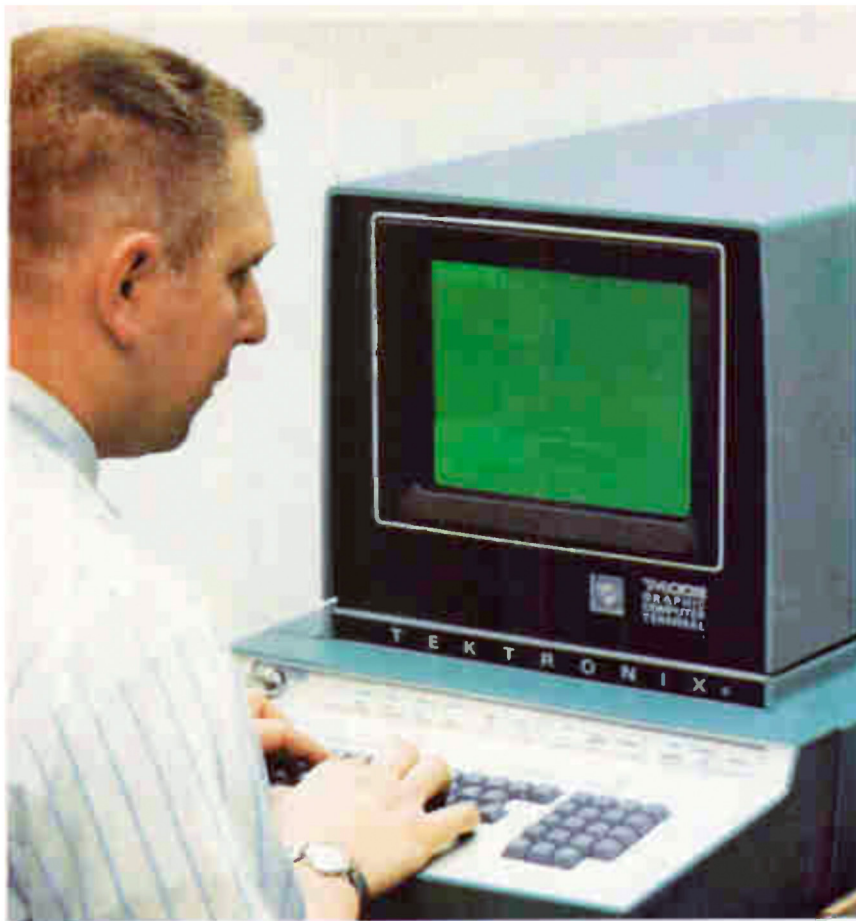
Loner. Terminal reads out alphanumeric and vectors, retains display without recycling of information by computer.
