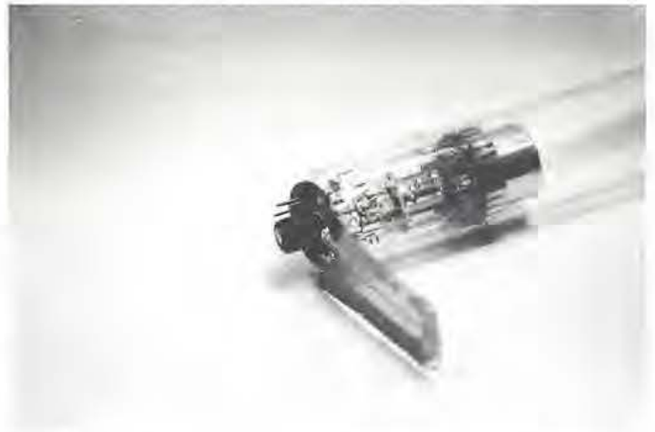
Fig. 2. VHR socket, gun, and transmission-line assembly.
