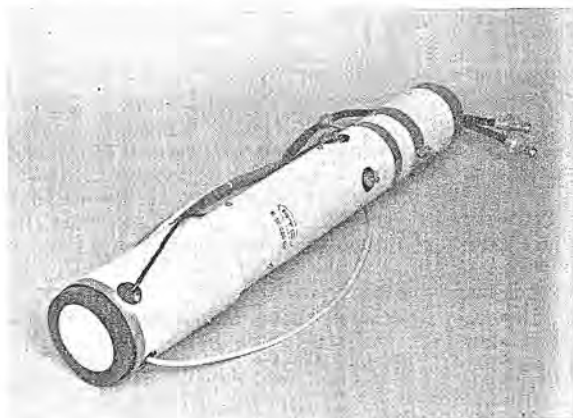
Figure 6 - TMC-5 Assembled with shield and cabling
