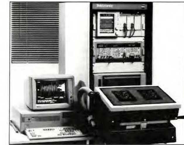
Fig 4. The test system seen here has a TDI 11400 scope, a TSA 8140 test system adapter (the apron) with a high-speed bed-of-nails fixture, and a TSI 8150 test system interface to control driver and scanner cards in the TSA. The system is controlled over a GPIB interface; here, desktop computer at left provides control.
