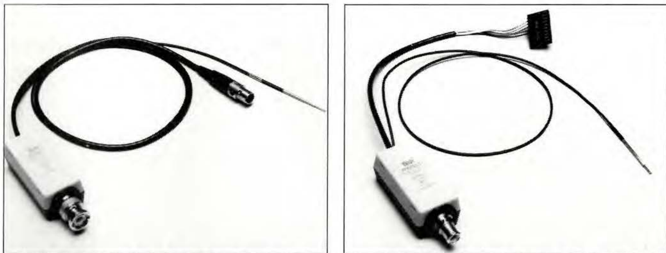
Fig 1. Like active probes used with high-frequency oscilloscopes, the 300-MHz P6511 (a) and P6513 (b) probes have a high input impedance (1 M \Omega and 3.8 pF) so as not to load a unit under test. But they're designed to fit in bed-of-nails fixtures, so they permit a new level of automated testing.
