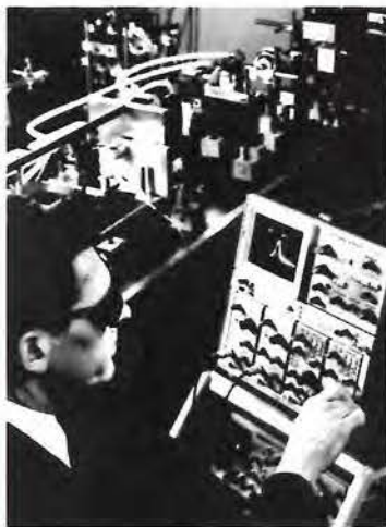
Though analog-storage scopes are still better for capturing high-speed, random, or single-shot signals, DSOs and digitizers are beginning to close the performance gap.
