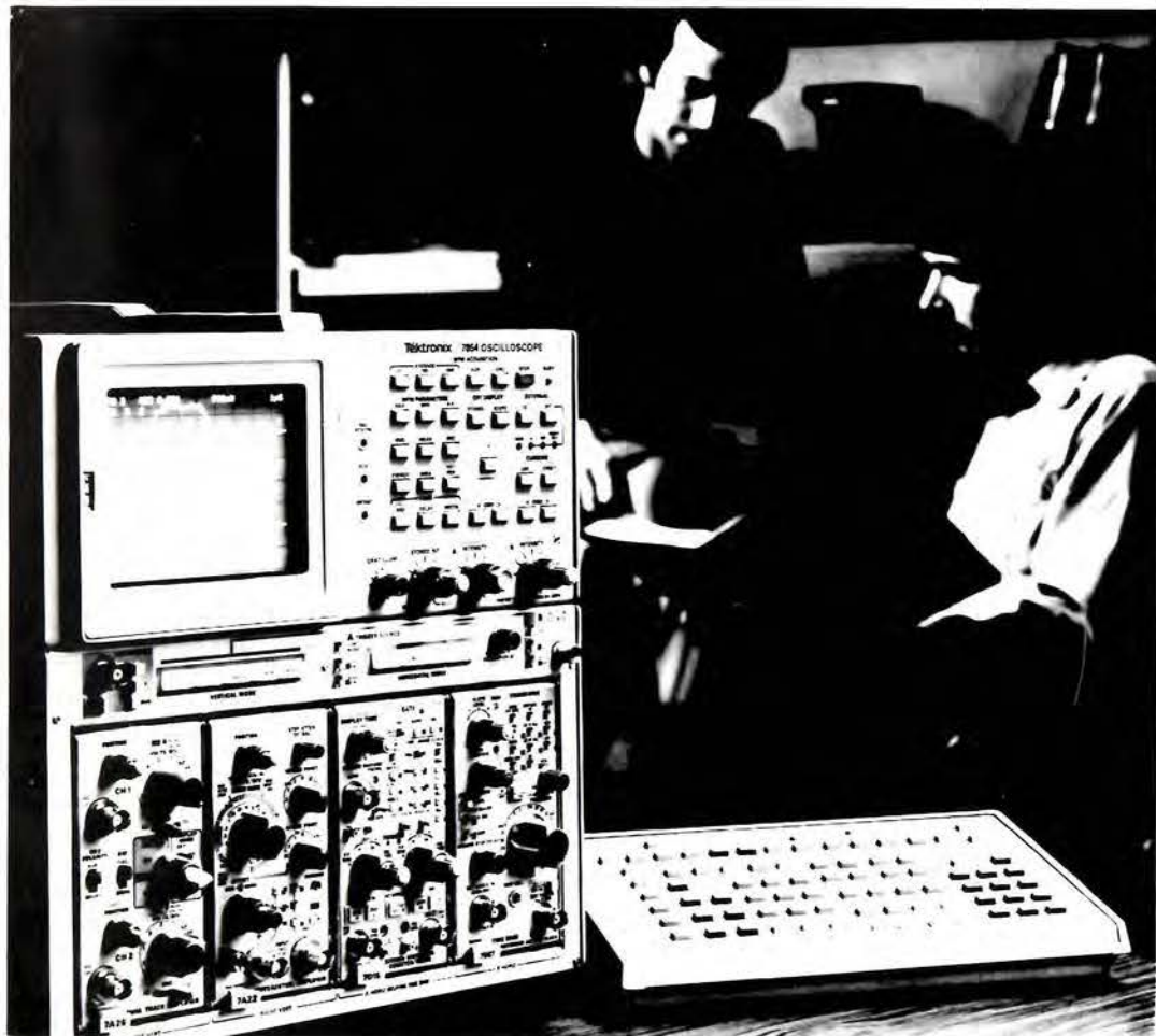
Tektronix's 7854 waveform processing oscilloscope is an example of the trend of combining processing power with programmability and the ability to be tailored to specific situations via plug-ins.
