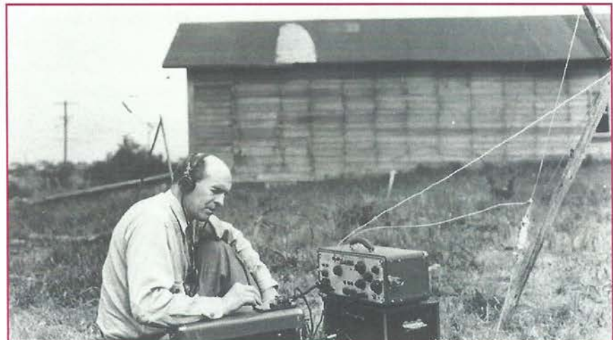
Forest Service radio pioneer Dwight Beatty operating his SP-1930 (Semi-Portable) Morse Code transceiver. Eight of these units were produced for fireline communications and testing. Photo: Forest Service, James Allen collection, Los Altos, CA.
