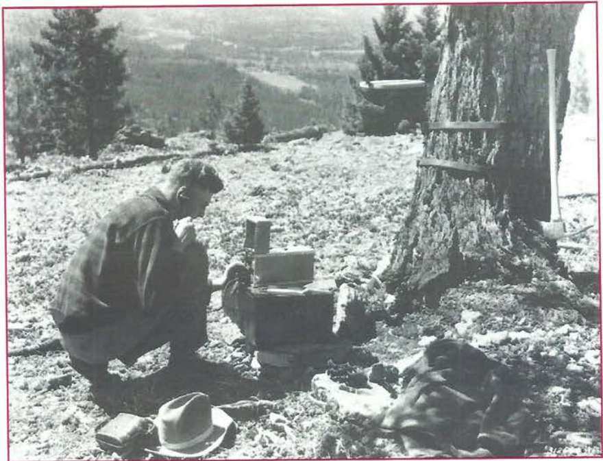
The Forest Service Type PF "Portable Fone" operated by Richard Ogg, Lolo National Forest, 1933. The PF was one of the smallest and lightest of the shortwave radio sets, so popular that some 450 were deployed by the Forest Service before it was replaced by an improved model in 1935. Photo: Forest Service.
