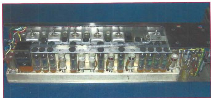
The Forest Service Type SF VHF-FM walkie-talkie, 1947. (Top right) Model A shown with its slide-out battery box. (Top left) Model C with external handset connector. (Below right) Inside the SF, showing its array of 27 tubes and intricate construction. More than 200 radio sets were made before commercial manufacturers began producing their own versions. Photo: Richard Ferranti.
