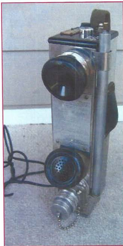
The Forest Service Type SF VHF-FM walkie-talkie, 1947. (Top right) Model A shown with its slide-out battery box. (Top left) Model C with external handset connector. (Below right) Inside the SF, showing its array of 27 tubes and intricate construction. More than 200 radio sets were made before commercial manufacturers began producing their own versions. Photo: Richard Ferranti.
