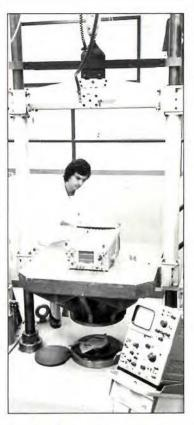
Two free fall shock machines are capable of testing a wide range of instrument sizes and weights. Accelerometers are available for monitoring shock response on the test item. Waveforms are stored in a digital oscilloscope.
