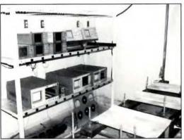
Testing facilities include an elevated temperature and humidity room and an elevated temperature room. Both have vibration machines and instrument power cycling equipment.
