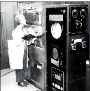
Programmable humidity chambers are capable of covering a wide range of temperature and humidity combinations.
