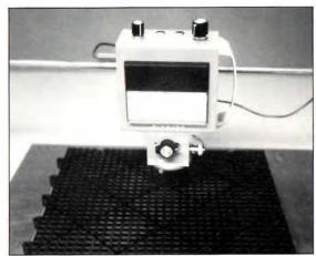
Surface resistance, static generation and static dis-sipation tests are performed on a wide range of materials and products.
