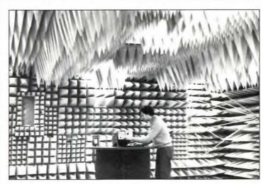
Electromagnetic emission testing for instruments or systems is conducted in our large anechoic chamber or open field site.
