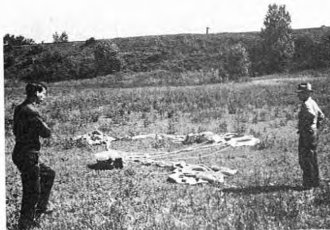
Figure 86. Parachute experiment with radio package. Note the loaves of bread on top of the package. One of a series of experiments conducted for Region 1 in the late 1930's to find a way of shock-proofing radios parachuted to smokejumpers on a fire. (Forest Service photo, History Section)
