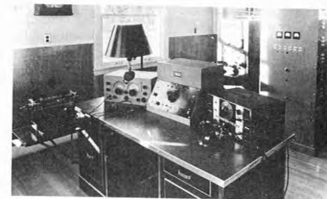
Figure 64. Transmitting and receiving equipment at the Radio Laboratory's Station KBAA, Portland, Ore. A new 250-watt transmitter installed about 1939 kept the Laboratory in close touch with personnel on field assignments. (Forest Service photo, History Section)
