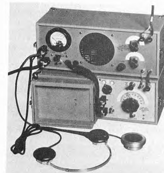
Figure 75. Type SX (superregenerative, crystal-controlled frequency) lower set, shown here interconnected for operation with the SXA, top. The SXA was an audio amplifier used as a standby speaker with the SX transceiver. The SX proved a very popular, light, portable set. It was a successor to the S and SV sets. See circuit diagram in appendix I. (NA:95G-407251)
