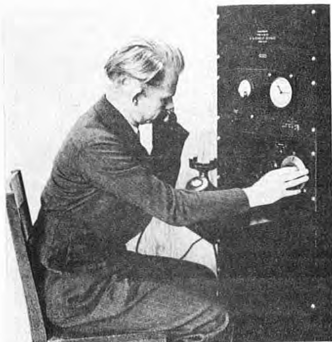
Figure 60. Logan Belleville, who designed it at the Radio Laboratory in 1936, is at the controls of a type U-30-25 fixed-base vhf radiophone with output power of 20 watts, in the Region 6 headquarters in Portland, Ore. (Forest Service photo, History Section).
