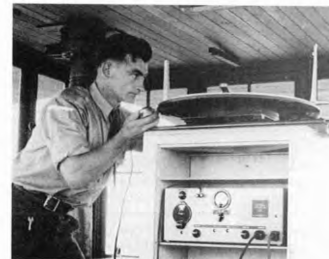
Figure 73. Type T, model D, located in base of fire finder, Pepper Lookout, Mt. Hood National Forest, Ore., July 1940. (NA:95G-397920)
