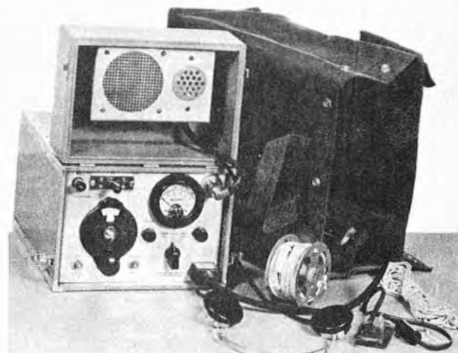
Figure 66. Front view of SPF model set up for portable use. (Forest Service photo, History Section)
