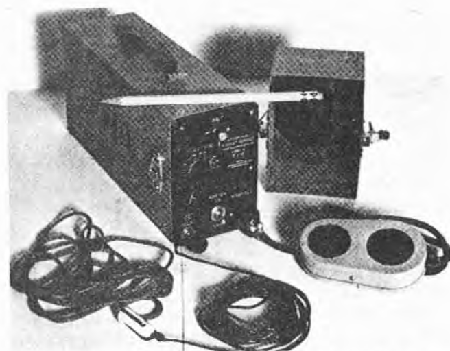
Figure 76. Type SJ set, developed as an ultralightweight model for smokejumpers, fitting into a special leg pocket and weighing only 6 pounds. Pencil gives an idea of its size. (Forest Service photo, History Section)
