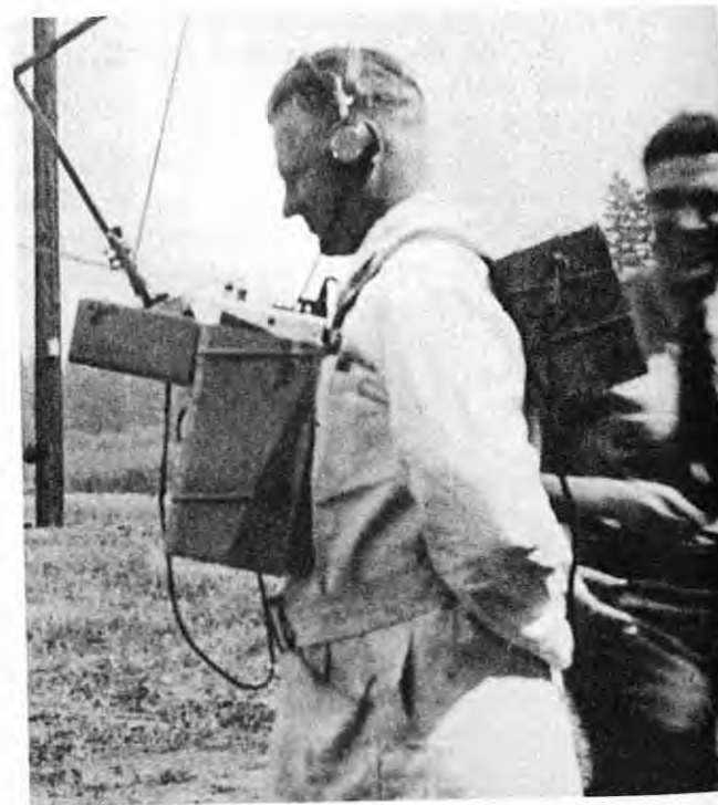
Figure 82. Ralph Kunselman demonstrates the experimental type X metal detector developed by the Radio Laboratory, while Harold Lawson looks on. The gadget was designed to warn sawyers of nails, bolts, spikes, wire, etc., in logs they were processing after the New England hurricane of 1938. The work came under the timber salvage program of the Forest Service and cooperating States. (Forest Service photo, History Section)
