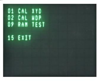
The interface firmware provides programs which are needed for proper calibration of the DPO. The programs are described in detail in the Tektronix manual "Checkout Software", 070-1612-00. Flowcharts can be found in the System and Calibration Manual, 070-1600-00.
