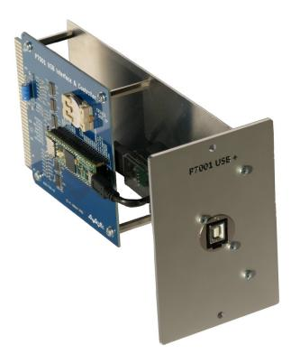
Optionally, the module can be equipped with an electrically isolated USB interface.
