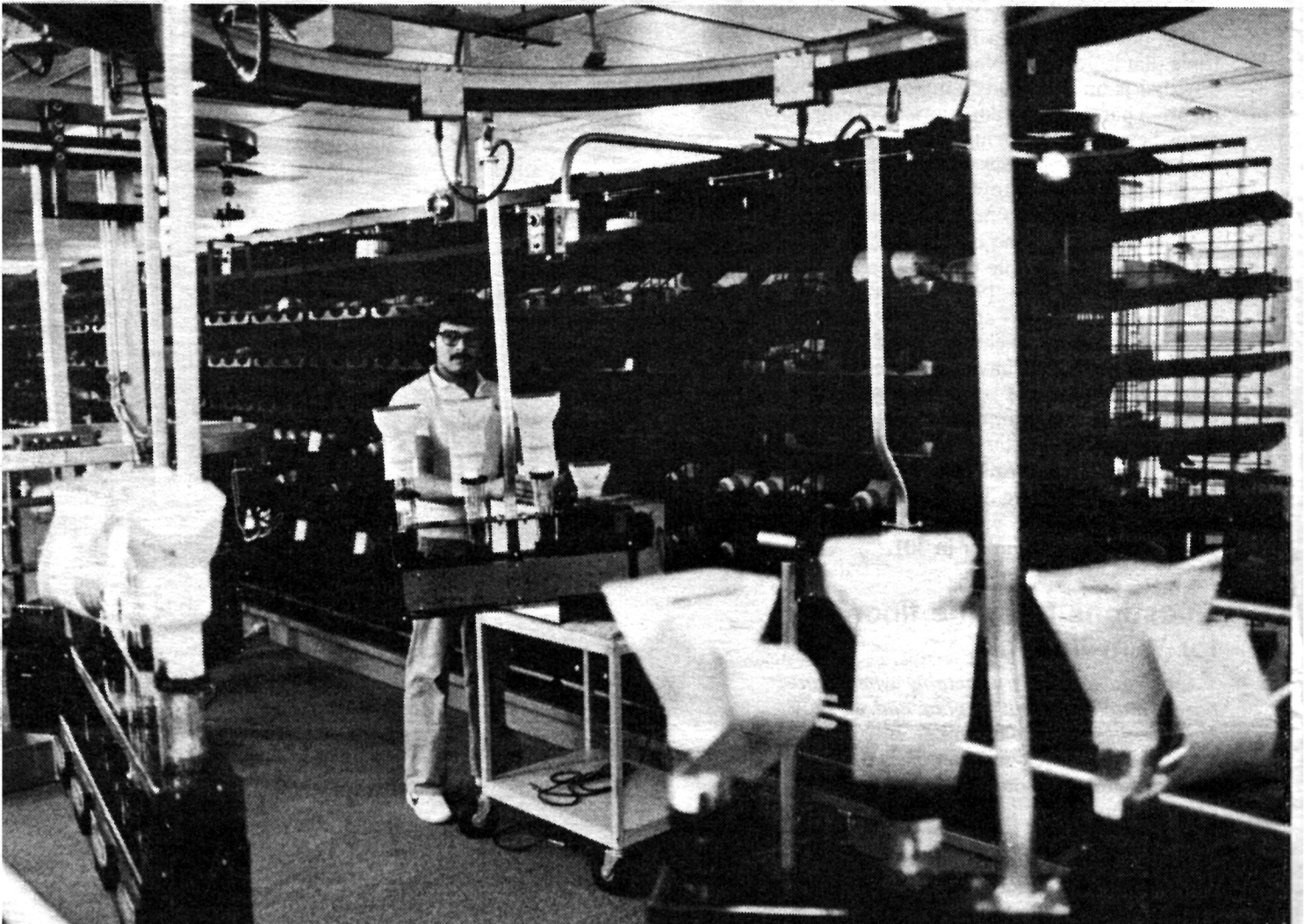
A MONORAIL runs throughout the high volume area to move CRT's from one work area to the next. Here, Joe Jimenez unloads CRT's from the activator monorail and places them in a carousel for distribution to test stations that are within an arm's reach of the carousel.
